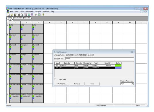
Insert the plate to begin the run and click the "Instrument" tab  $\rightarrow$  "Start".
