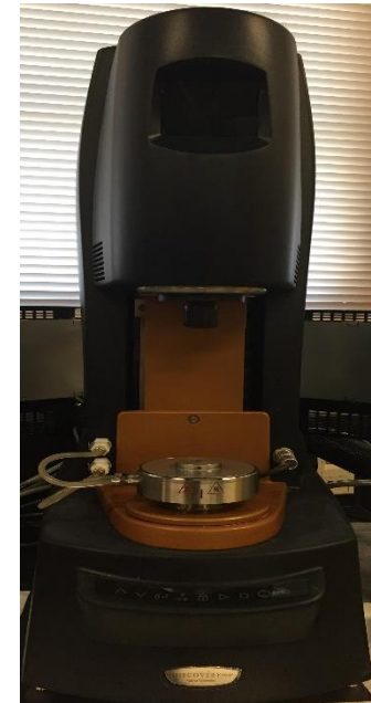
TA Instruments HR2 rheometer with solvent trap
