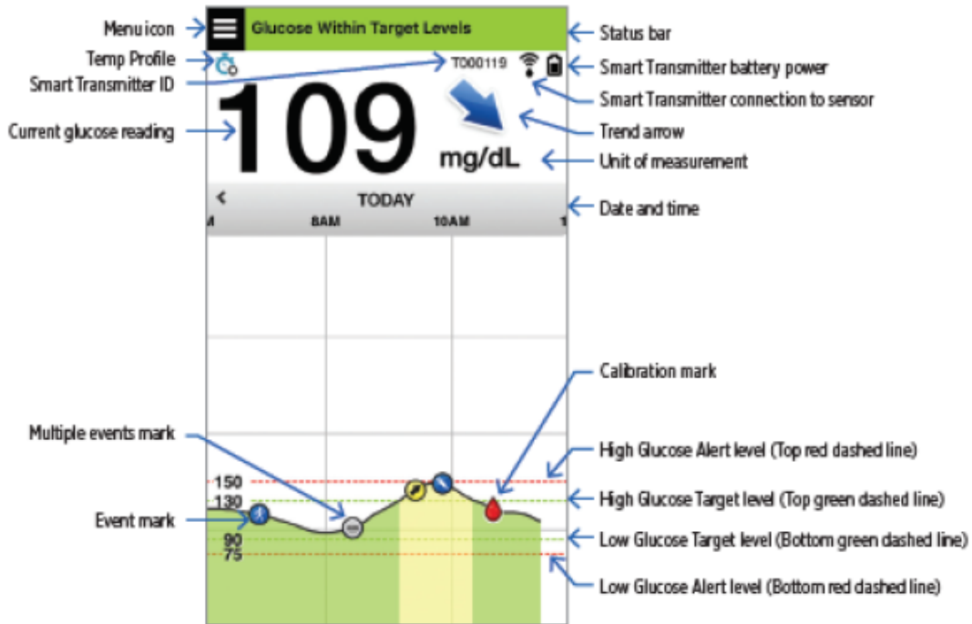
Figure 1 - Eversense CGM display. The status bar reports the current, real-time glucose value as well as a trend arrow, whose direction informs the user about the glucose trend direction and rate (i.e., glucose is 109 mg/dL and dropping in this example). The glucose information window provides the glucose trace graph (tracking information) for the previous several hours.
