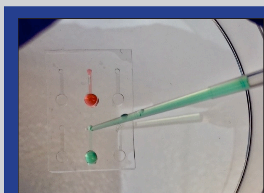
Demonstration of sample solutions being pipetted into channel opening (small opening at the left side of the channel) and moving under pressure to reservoir (large opening at the right side of a channel). The small bore of the channel provides an environment that is more confined than are open wells in plastic dishes.
