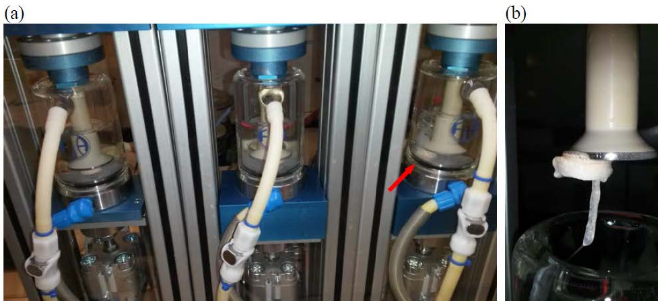
Figure 4: Images of Erweka DRT chewing machine (a) during the chewing cycles and (b) at the end of chewing study (Study report from the OPQ/ OTR)
