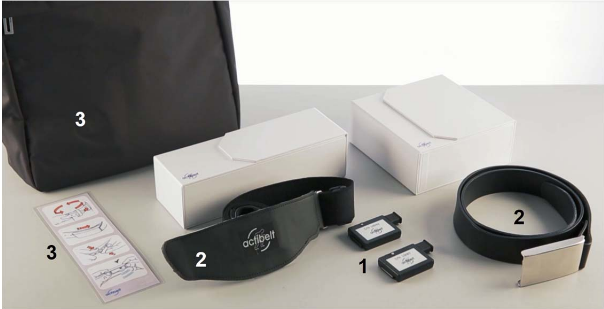
Figure 3-1 actibelt unit components
