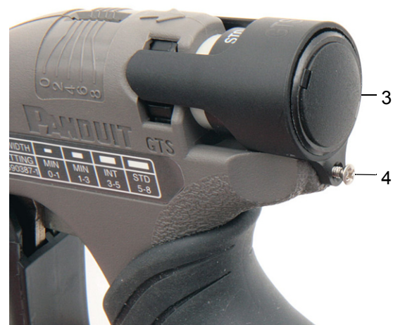
Fig. 5-5 Assemble the locking cap
