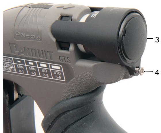
Fig. 5-3 Disassemble the locking cap
