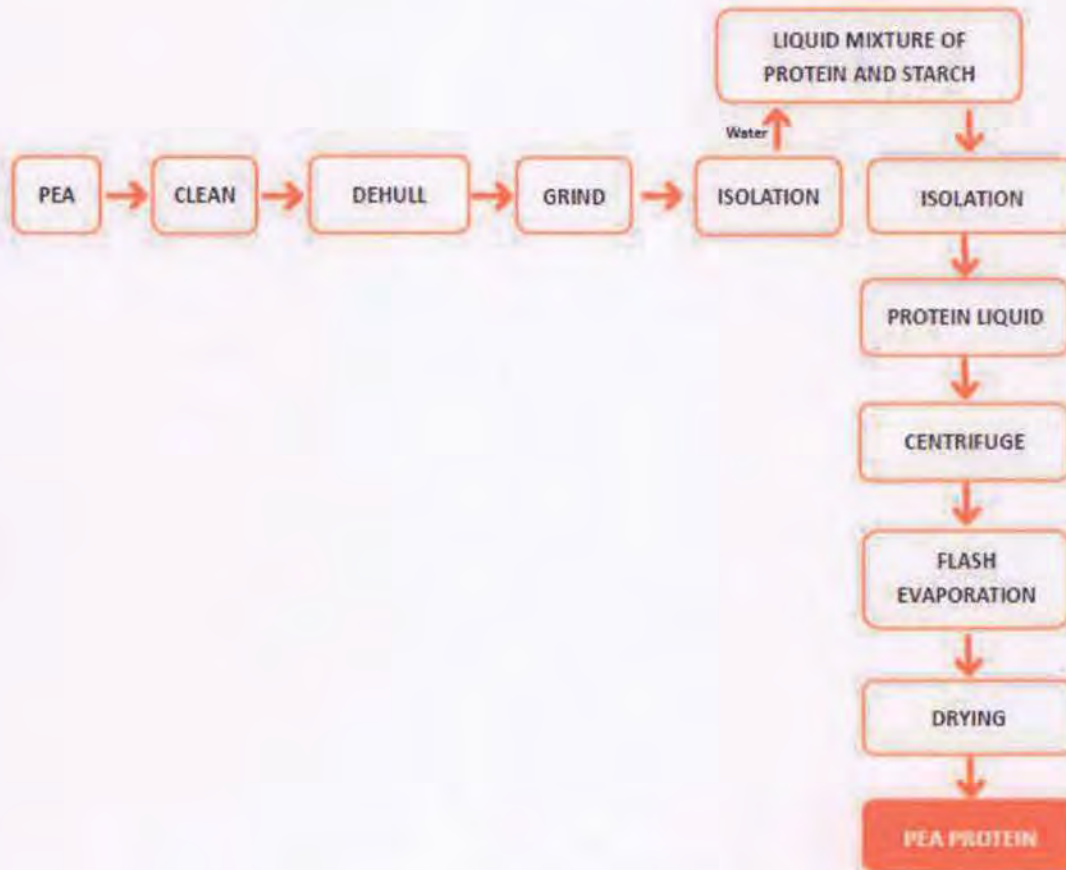
Figure 2. Manufacturing Process of Pea Protein
