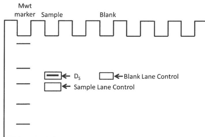
**Figure 1b:** Diagram of a gel showing how a user defined the UDR's which will give the Total Densities for the Band ( $D_s$ ), a Sample Lane Control ( $D_{SLC}$ ) and the Blank Lane Control ( $D_{BLC}$ ).
