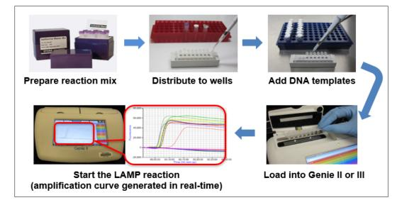
**IMPORTANT**: Before starting to assemble a LAMP reaction on the bench, first set up a new LAMP run and enter sample information on Genie instruments or 7500 Fast (see **Section E.1 or E.2**, **respectively, through step c**).
