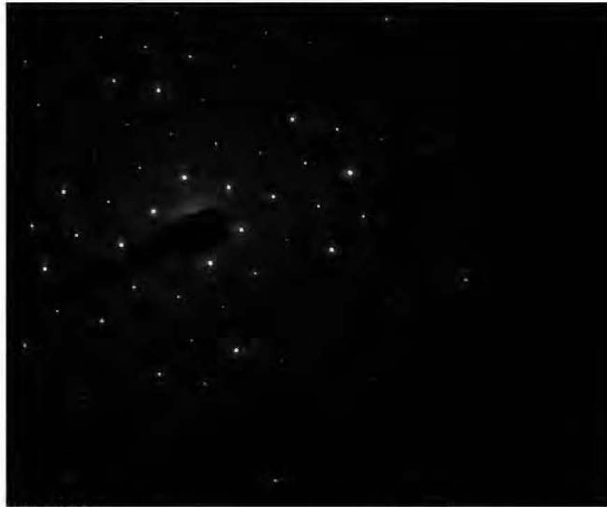
Hexagonal Diffraction Pattern from Talc Particle pictured above
