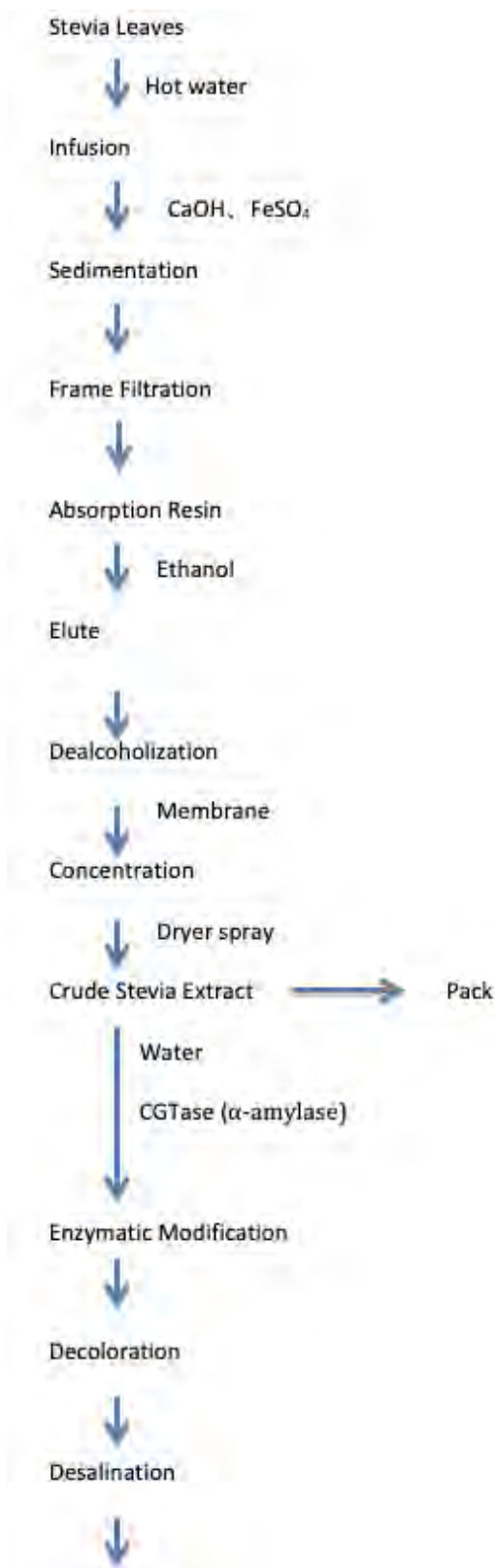
Figure 3. Flow Chart of Manufacturing Process for Qufu, Sunwin, and NuNaturals’s TasteRight High Purity Glucosylated Steviol Glycosides Preparations
