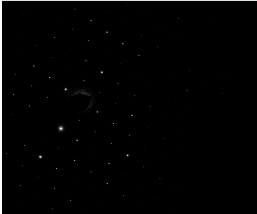
300396 FDA_003.jpg Mica Particle Diffraction Spectra 1 09:46 4/2/2019 Microscopist: (b) (4) Camera: (b) (4) Exposure: 800 (ms) x 5 drift frames, Gain: 1, Bin: 1 Gamma: 1.00, No Sharpening, Normal Contrast 100 (1/Å) HV=100kV Cam Len: 0.2200 m AMA Analytical Services, Inc
