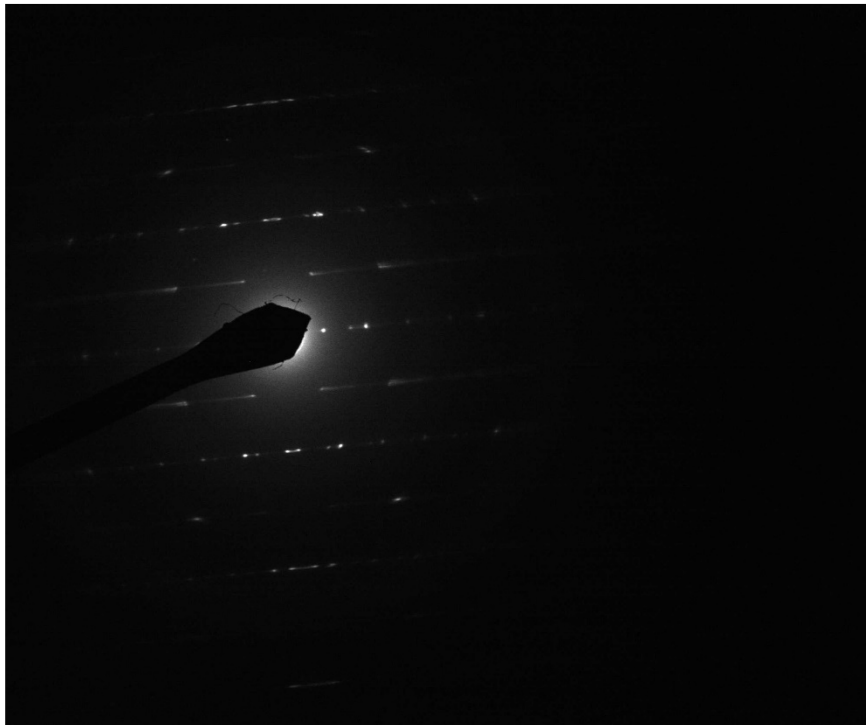
300396 FDA_118.jpg Chry Diff 5 11:51 4/16/2019 Microscopist: (b) 100 (1/Å) HV=100kV Cam Len: 0.2200 m AMA Analytical Services, Inc Camera: NANOSPRT5, Exposure: 800 (ms) x 5 drift frames, Gain: 1, Bin: 1 Gamma: 1.00, No Sharpening, Normal Contrast
