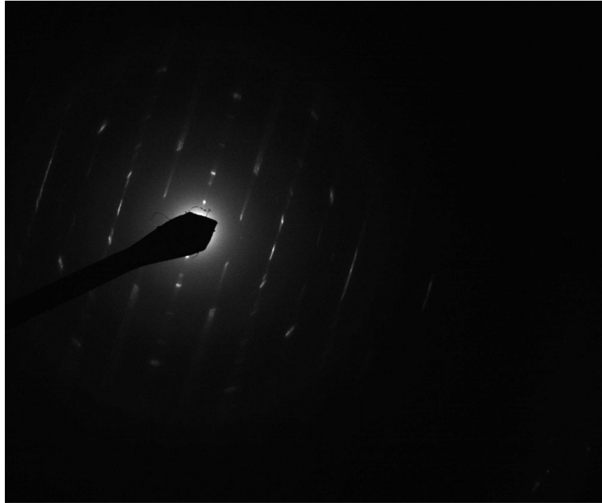
Sample 300396-4A Diffraction pattern from chrysotile structure #2 pictured above.
