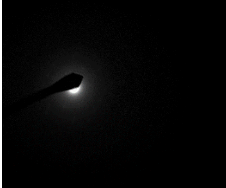
Sample 3b_002.tif Sample 3B Structure 3 3.9 x 0.1 Chrysotile Diffraction 10:21 4/18/2019 Microscopist: (b) (6) Camera: NANOSPRT5, Exposure: 800 (ms) x 5 drift frames, Gain: 1, Bin: 1 Gamma: 1.00, No Sharpening, Normal Contrast 100 (1/Å) HV=100kV Cam Len: 0.2200 m AMA Analytical Services, Inc
