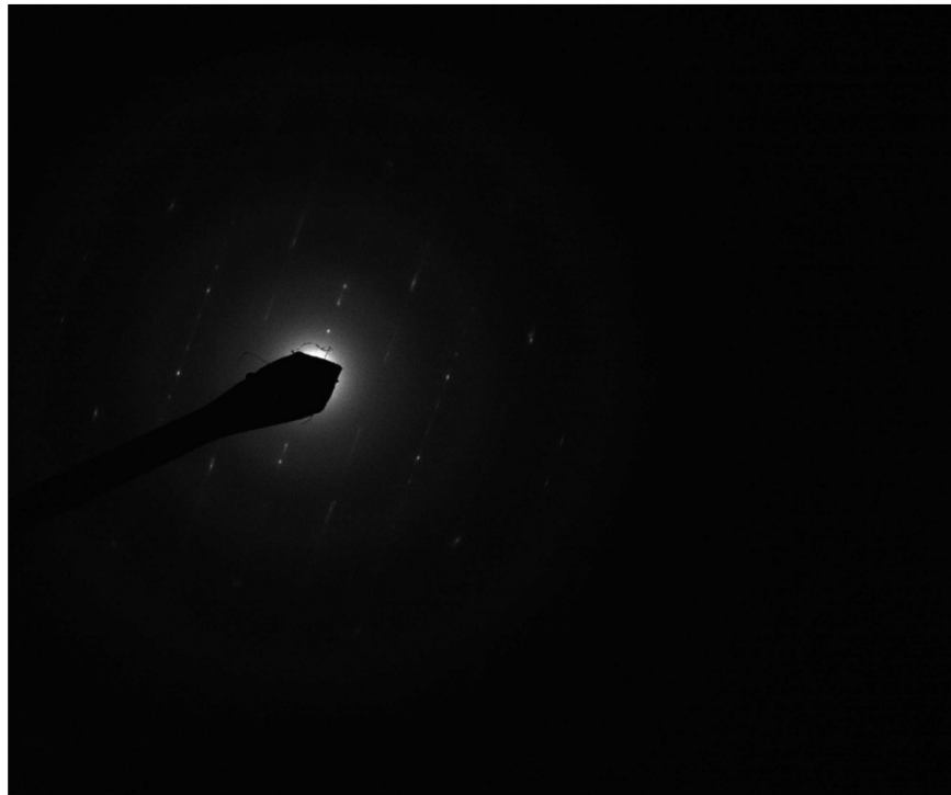
300396 FDA_107.jpg Chrysotile Diffraction 10:45 4/16/2019 Microscopist: (b) 100 (1/Å) HV=100kV Cam Len: 0.2200 m AMA Analytical Services, Inc Camera: NANOSPRT5, Exposure: 800 (ms) x 5 std. frames, Gain: 1, Bin: 1 Gamma: 1.00, No Sharpening, Normal Contrast
