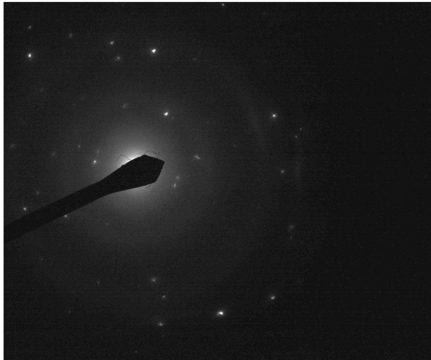
300396 FDA_007.jpg Titanium Dioxide Diffraction Spectra 10 10:02 4/2/2019 Microscopist: [b] Camera: NANOSPRT5, Exposure: 800 (ms) x 5 drift frames, Gain: 1, Bin: 1 Gamma: 1.00, No Sharpening, Normal Contrast 100 (1/Å) HV=100kV Cam Len: 0.2200 m AMA Analytical Services, Inc
