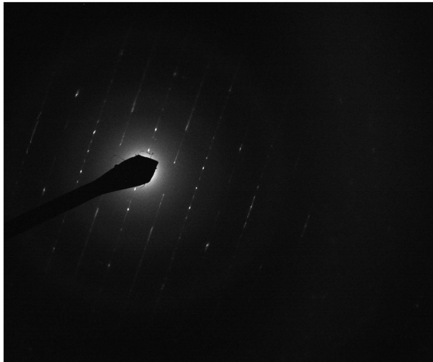
300396 FDA_113.jpg Chry Diff 3 11:02 4/16/2019 Microscopist: (b) 100 (1/Å) HV=100kV Cam Len: 0.2200 m AMA Analytical Services, Inc Camera: NANOSPRT5, Exposure: 800 (ms) x 5 drift frames, Gain: 1, Bin: 1 Gamma: 1.00, No Sharpening, Normal Contrast
