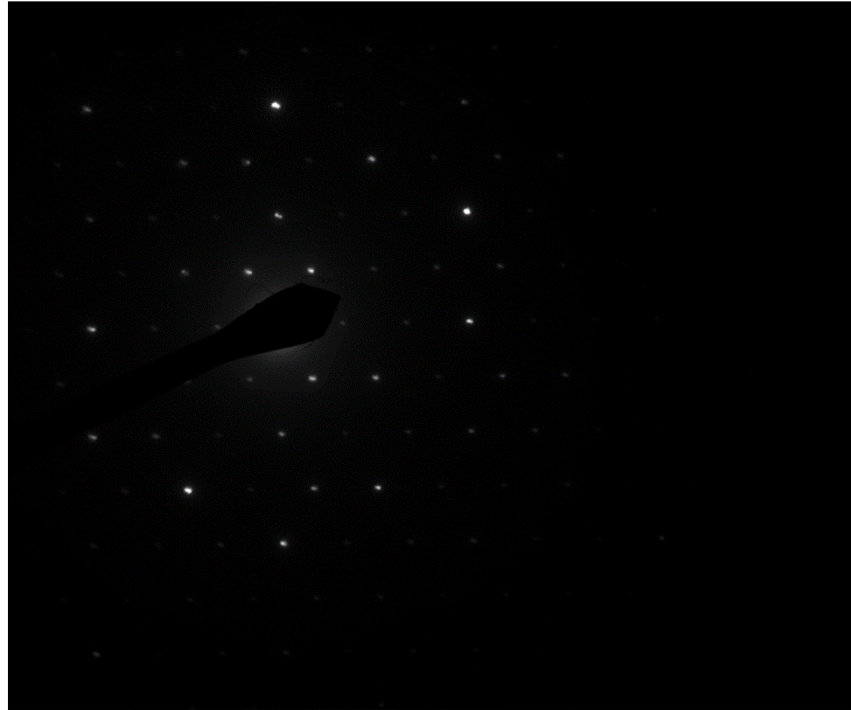
Sample 300396-7A Diffraction pattern from talc fiber pictured above.
