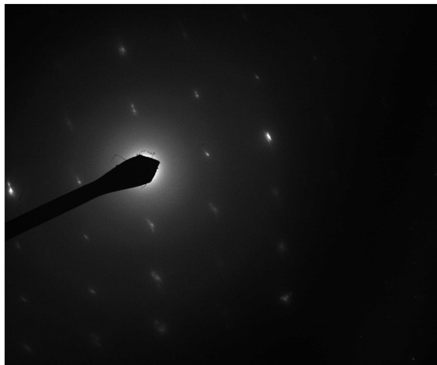
300396 FDA_033.jpg Talc Ribbon Diff 14:37 4/4/2019 Microscopist: [b] Camera: NANOSPRT5, Exposure: 800 (ms) x 5 drift frames, Gain: 1, Bin: 1 Gamma: 1.00, No Sharpening, Normal Contrast 100 (1/Å) HV=100kV Cam Len: 0.2200 m AMA Analytical Services, Inc
