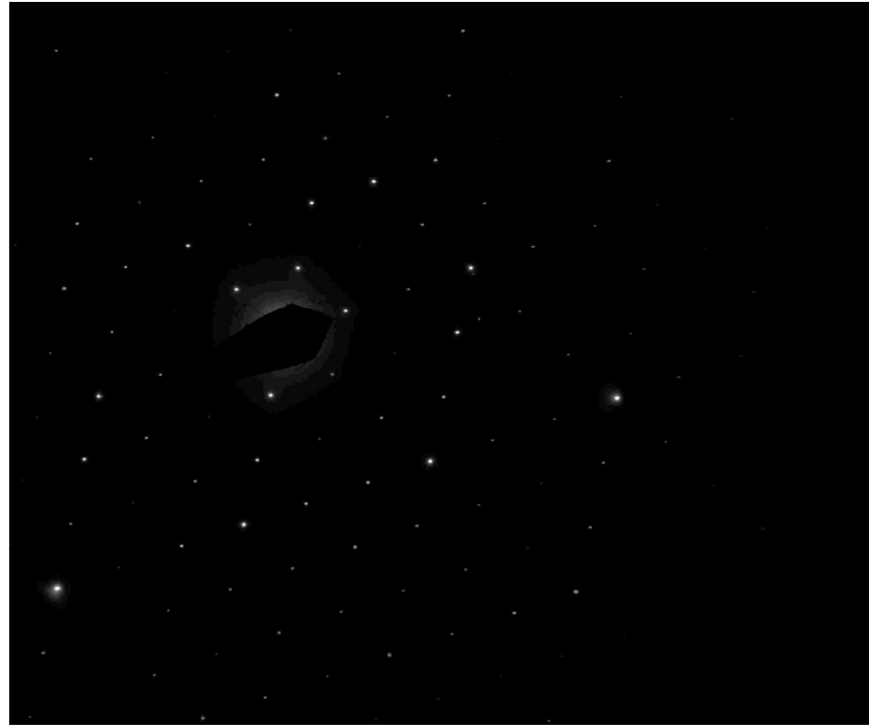
Sample 300396-2 Hexagonal diffraction pattern from mica particle pictured above.
