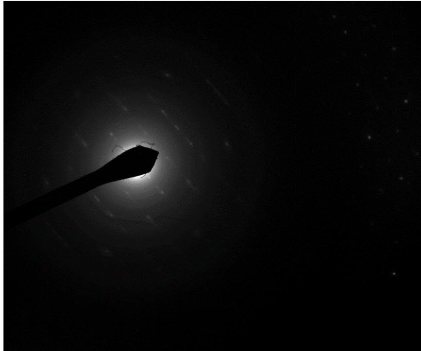
Sample 300396-3A Diffraction pattern from the chrysotile structure pictured above.
