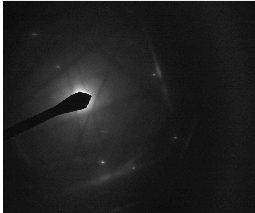
Sample 300396-1 Diffraction pattern from titanium particle pictured above.
