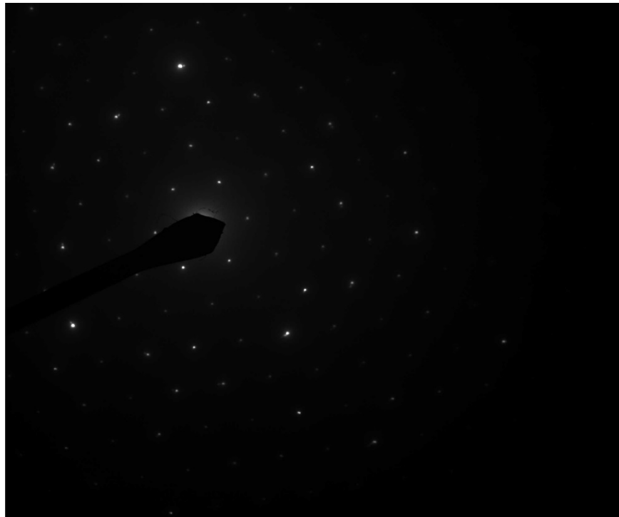
Hexagonal diffraction from the Talc particle pictured above.
