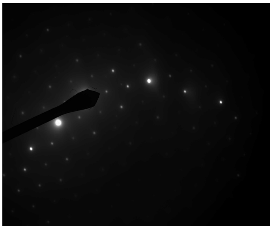
Diffraction pattern from the Mica particle pictured above.
