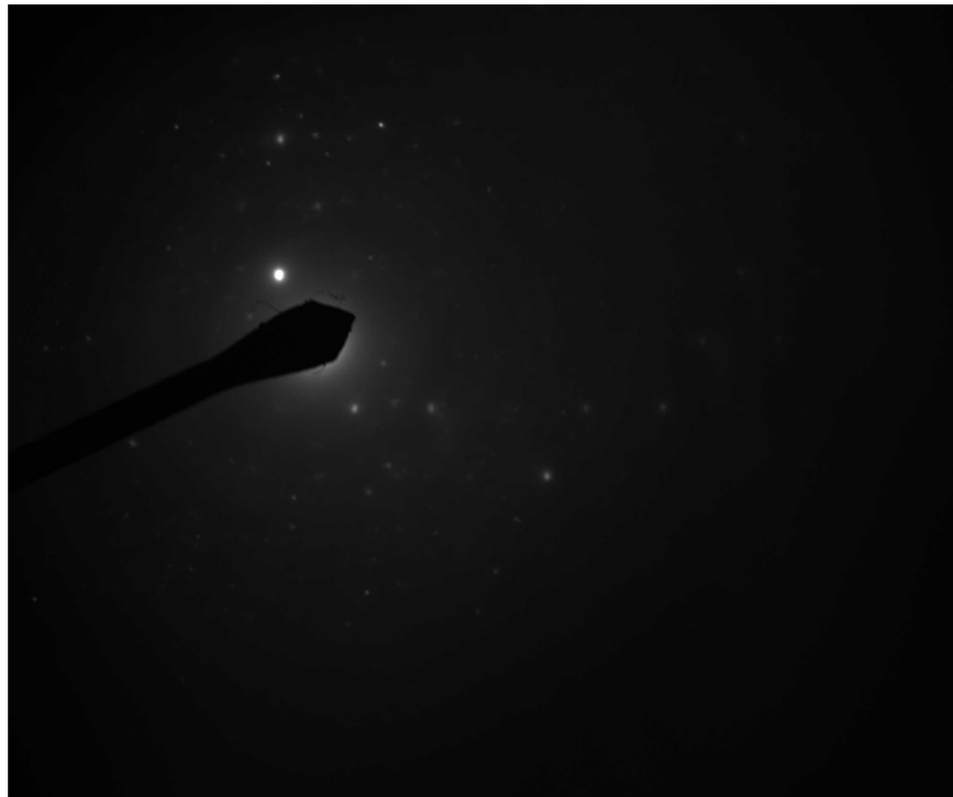
308006 FDA_011.jpg Titanium Coated Particle 14:47 8/21/2019 TEM Mode: Diffraction Microscopist: (b) Camera: NANOSPRT5, Exposure: 800 (ms) x 5 std. frames, Gain: 1, Bin: 1 Gamma: 1.00, No Sharpening, Normal Contrast
