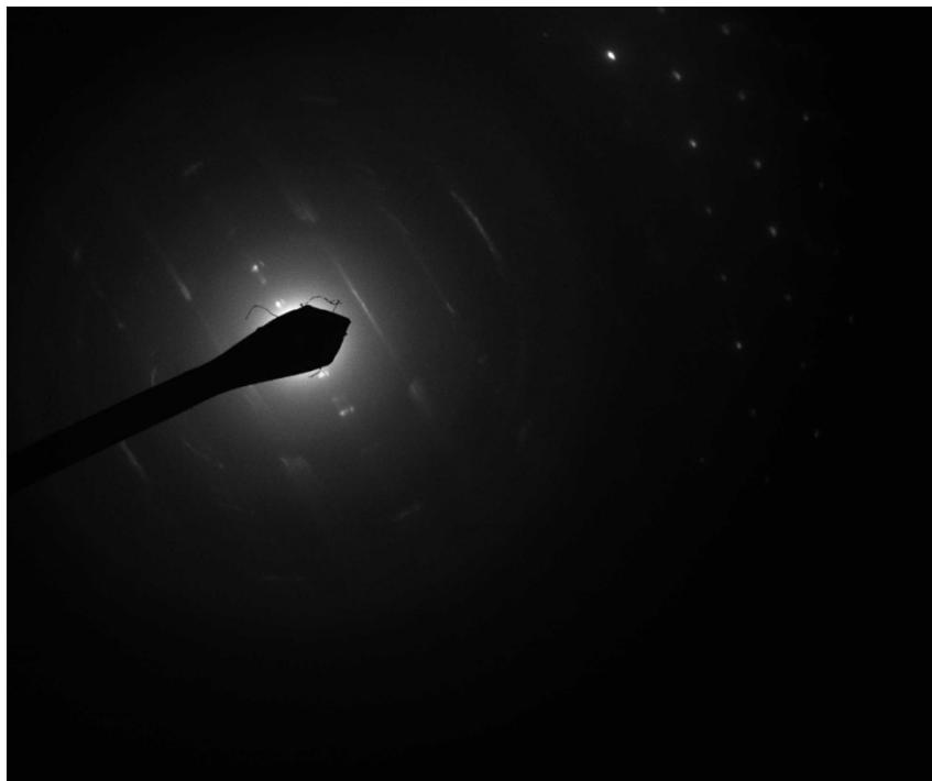
308006 FDA_104.jpg Chrysotile Dif 308006-6b 16:03 9/7/2019 TEM Mode: Diffraction Microscopist: (b) (6) Camera: NANOSPRT5, Exposure: 800 (ms) x 5 std. frames, Gain: 1, Bin: 1 Gamma: 1.00, No Sharpening, Normal Contrast 100 (1/Å) HV=100kV Cam Len: 0.2200 m AMA Analytical Services, Inc
