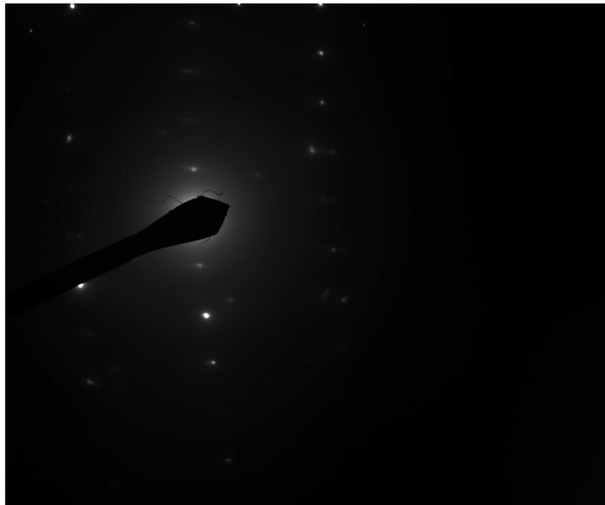
308006 FDA_019.jpg Possible Mica 15:31 8/21/2019 TEM Mode: Diffraction Microscopist: (b) Camera: NANOSPRT5, Exposure: 800 (ms) x 5 drift frames, Gain: 1, Bin: 1 Gamma: 1.00, No Sharpening, Normal Contrast
