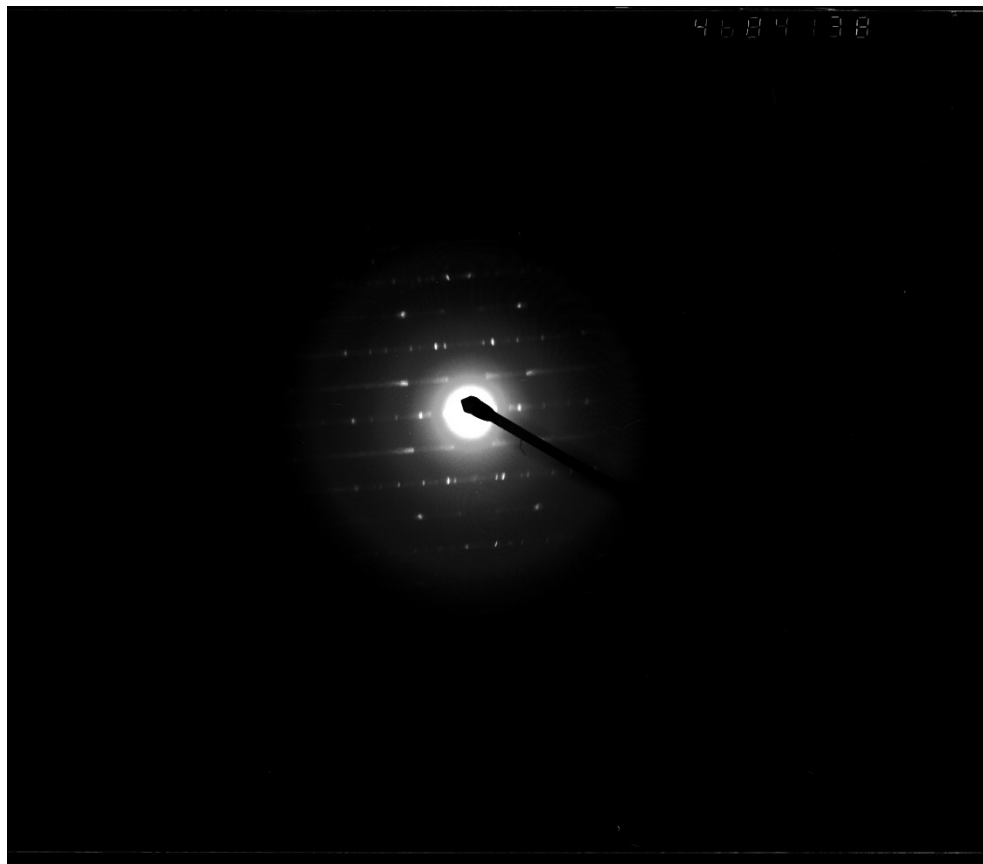
Diffraction pattern from the Chrysotile structure pictured above. (the image below was taken on film; the digital version was scanned from a negative)
