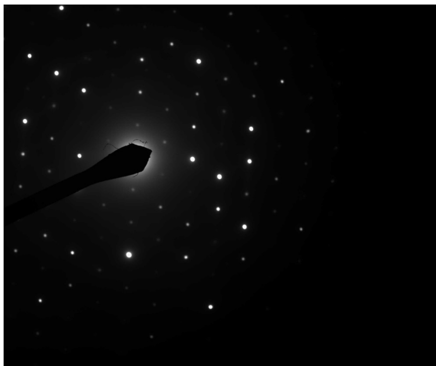
310123 FDA_026.jpg Mica Particle 17:14 9/18/2019 TEM Mode: Diffraction Microscopist: (b) Camera: NANOSPRT5, Exposure: 800 (ms) x 5 drift frames, Gain: 1, Bin: 1 Gamma: 1.00, No Sharpening, Normal Contrast
