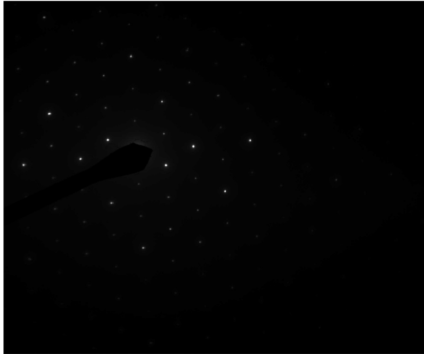
Diffraction pattern from the Talc Fiber pictured above
