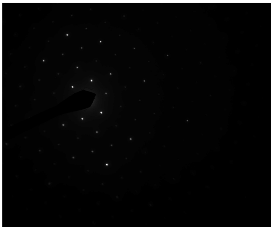
310123 FDA_084.jpg Talc Particle 12:21 9/22/2019 TEM Mode: Diffraction Microscopist: (b) Camera: NANOSPRT5, Exposure: 800 (ms) x 5 drift frames, Gain: 1, Bin: 1 Gamma: 1.00, No Sharpening, Normal Contrast
