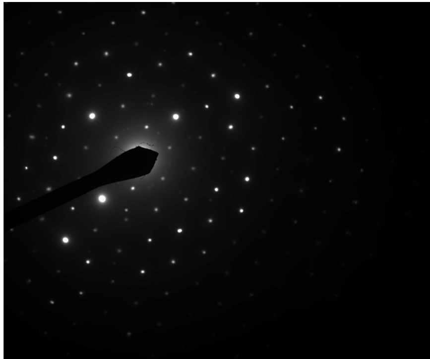
310123 FDA_071.jpg Mica Particle 11:16 9/22/2019 TEM Mode: Diffraction Microscopist: (b) (6) Camera: NANOSPRT5, Exposure: 800 (ms) x 5 drift frames, Gain: 1, Bin: 1 Gamma: 1.00, No Sharpening, Normal Contrast
