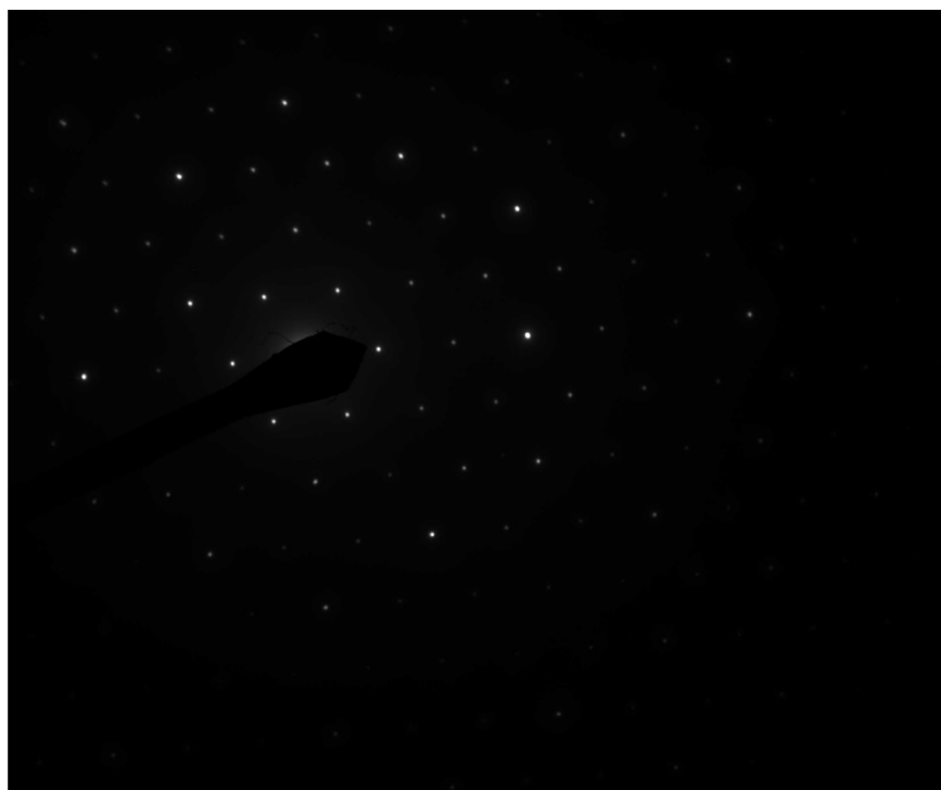
310123 FDA_123.jpg Talc Fiber 13:34 9/25/2019 TEM Mode: Diffraction Microscopist: (b) (6) Camera: NANOSPR5, Exposure: 800 (ms) x 5 drift frames, Gain: 1, Bin: 1 Gamma: 1.00, No Sharpening, Normal Contrast
