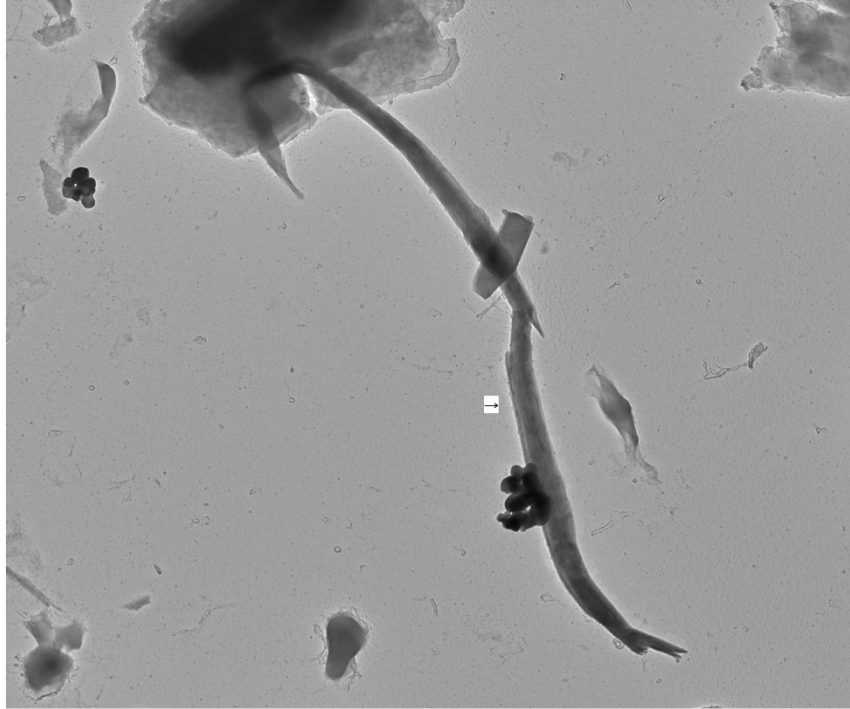
310123 FDA_136.jpg Talc Ribbon Cal: 0.003548 \mu\text{m}/\text{pix} 15:15 9/25/2019 TEM Mode: Imaging Microscopist: (b) Camera: NANOSPRT5, Exposure: 800 (ms) x 5 drift frames, Gain: 1, Bin: 1 Gamma: 1.00, No Sharpening, Normal Contrast
