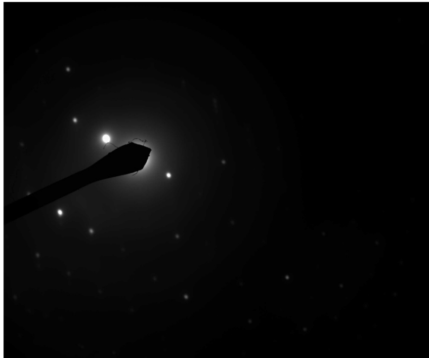
310123 FDA_020.jpg Non Asbestos Particle 15:57 9/18/2019 TEM Mode: Diffraction Microscopist: (b) [redacted] Camera: NANOSPRT5, Exposure: 800 (ms) x 5 drift frames, Gain: 1, Bin: 1 Gamma: 1.00, No Sharpening, Normal Contrast
