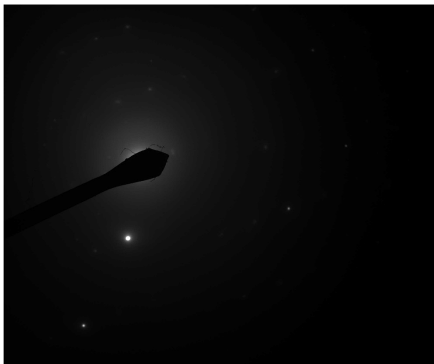
Diffraction pattern from the Silica Particle pictured above.
