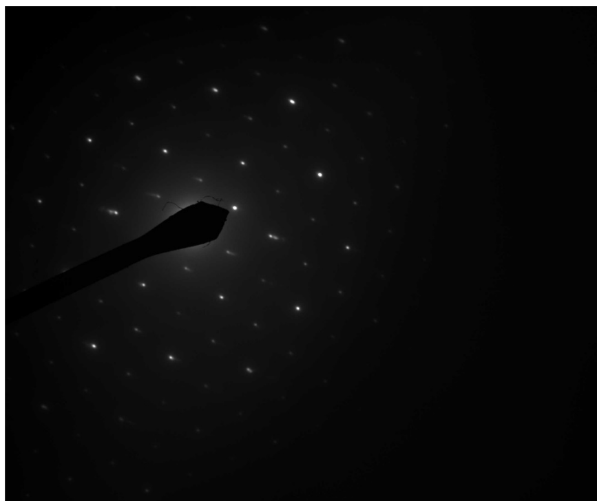
310123 FDA_036.jpg Talc Particle 10:30 9/19/2019 TEM Mode: Diffraction Microscopist: (b) Camera: NANOSPRT5, Exposure: 800 (ms) x 5 drift frames, Gain: 1, Bin: 1 Gamma: 1.00, No Sharpening, Normal Contrast
