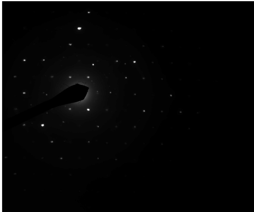
310123 FDA_065.jpg Mica Fiber 10:14 9/22/2019 TEM Mode: Diffraction Microscopist: (b) Camera: NANOSPRT5, Exposure: 800 (ms) x 5 drift frames, Gain: 1, Bin: 1 Gamma: 1.00, No Sharpening, Normal Contrast
