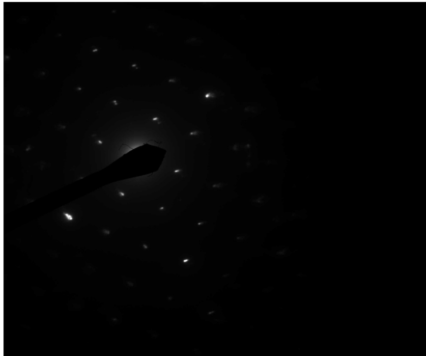
310123 FDA_137.jpg Talc Ribbon 15:16 9/25/2019 TEM Mode: Diffraction Microscopist: (b) Camera: NANOSPRT5, Exposure: 800 (ms) x 5 drift frames, Gain: 1, Bin: 1 Gamma: 1.00, No Sharpening, Normal Contrast
