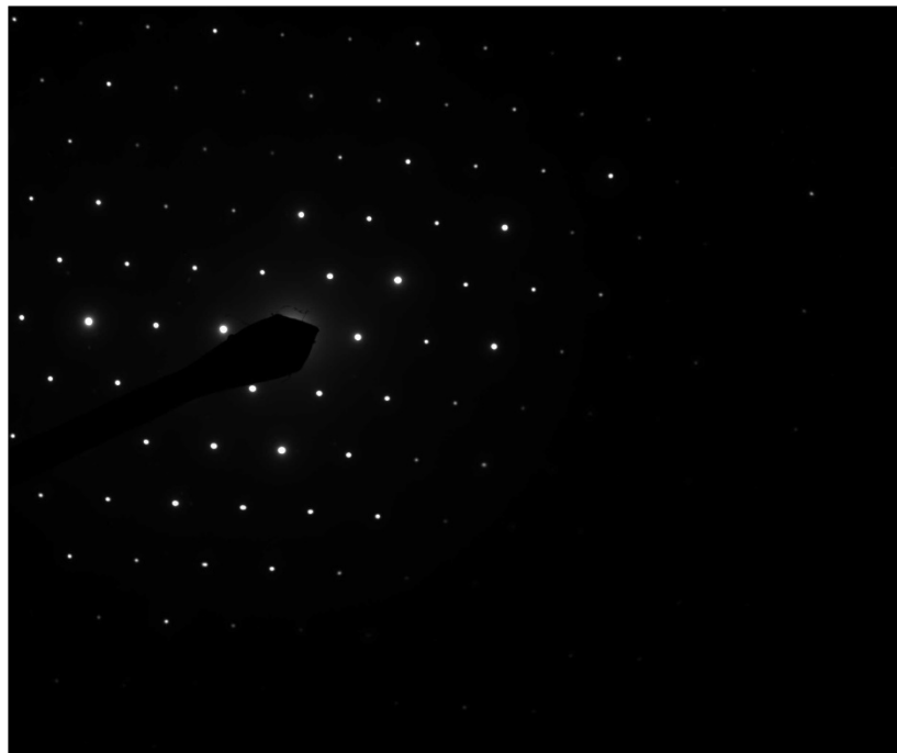
310123 FDA_002.jpg Mica Particle 14:50 9/18/2019 TEM Mode: Diffraction Microscopist: (b) Camera: NANOSPRT5, Exposure: 800 (ms) x 5 drift frames, Gain: 1, Bin: 1 Gamma: 1.00, No Sharpening, Normal Contrast
