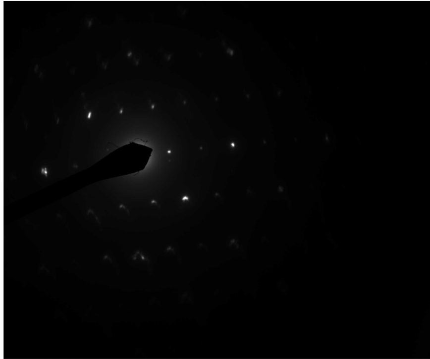
Hexagonal diffraction pattern from the Talc Fiber pictured above
