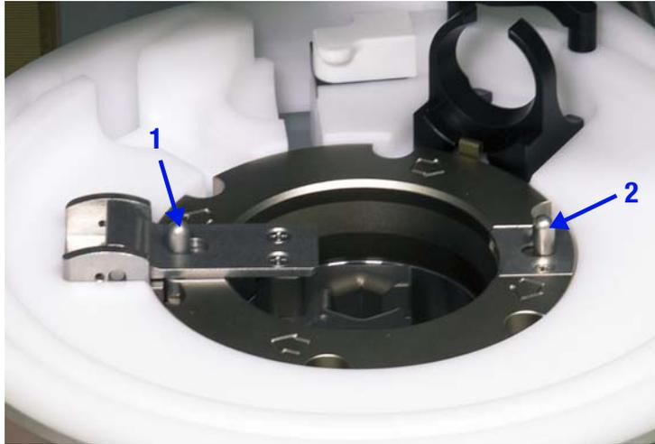
**Figure 5-1:** Location of the filler latch pin (1) and the filler locking pin (2)
