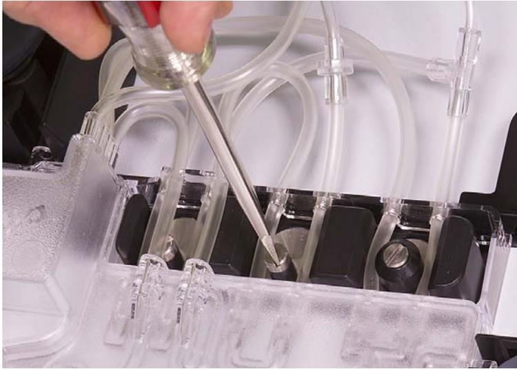
**Figure 16-8:** Valves turned to the neutral position
