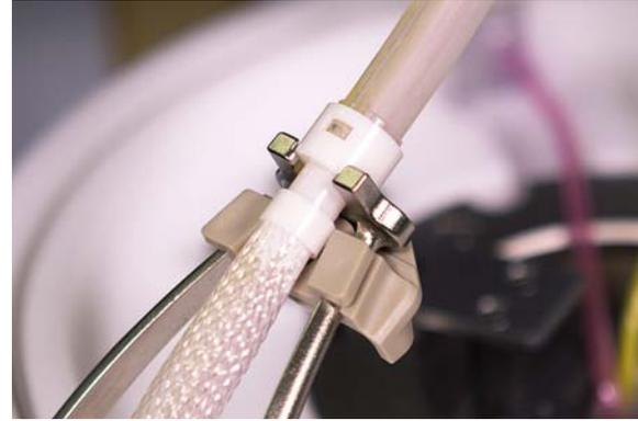
**Figure 5-9:** Upper bearing inserted in the upper bearing holder
