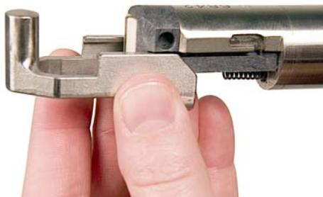
**Figure 17-6:** Aligning the jaw with the grooves
