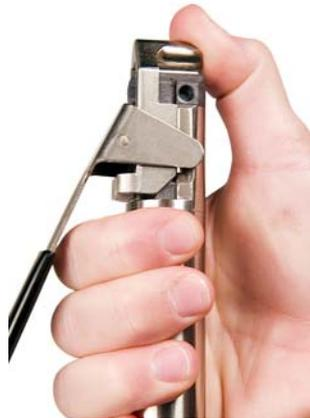
**Figure 17-3:** Depressing the jaw to the closed position
