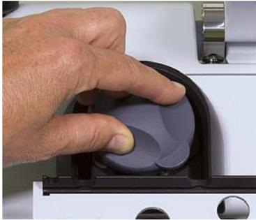
**Figure 17-1:** Removing the rotor from the pump housing
