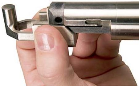
**Figure 17-5:** Removing the jaw
