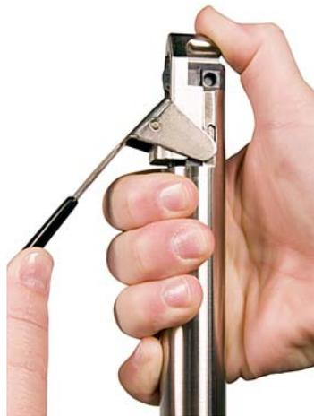
**Figure 17-7:** Replacing the lever
