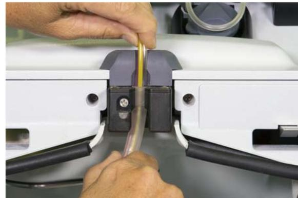
**Figure 5-11:** Upper collar secured in the upper collar holder
