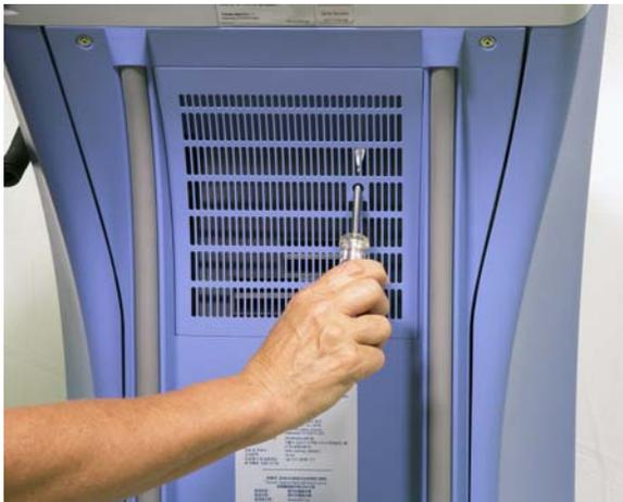
**Figure 16-9:** Screwdriver inserted in the hole in the back of the system
