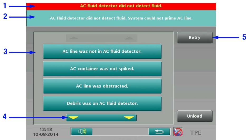
Figure 16-1: Example of an active alarm screen
