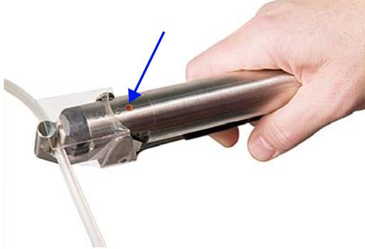
**Figure 15-2:** Hold the jaw closed until the indicator light illuminates
