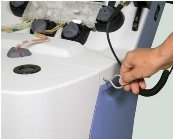
**Figure 16-7:** Centrifuge door key in the lock-release hole
