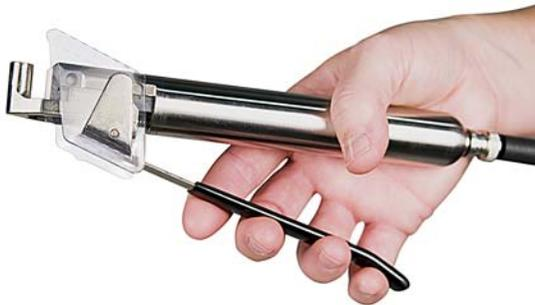
**Figure 15-1:** Hold the sealer head with jaws open facing upward
