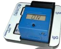
Press the button again; the display will read "RFID". Place the DPP COVID-19 IgM/IgG RFID card on top of the reader and a beep will sound.
