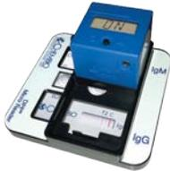
Press the button again; the display will read "RFID". Place the DPP COVID-19 IgM/IgG RFID card on top of the reader and a beep will sound.
