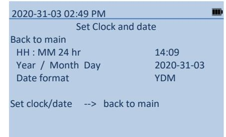
5 After setting the clock and date, hold the button down for >1 second to go "back to main" screen.
