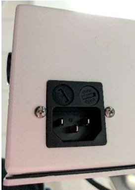
LCU Power Receptacle – underside of LCU stimulation electronics enclosure
