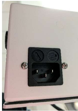
LCU Power Receptacle (on the underside of the LCU)
