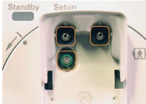
O-rings in the water trap holder
