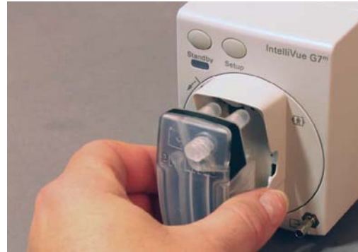
Installing the water trap
