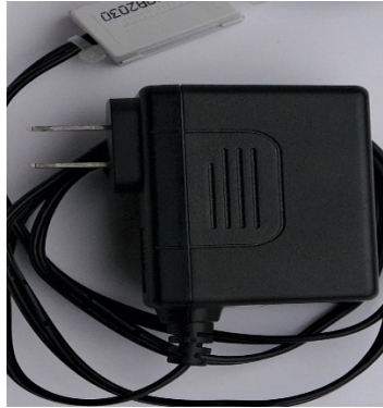
Figure 34. External AC/DC Converter
