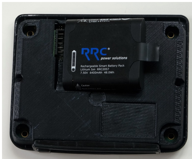
Figure 38: VentFree battery with pull tab
