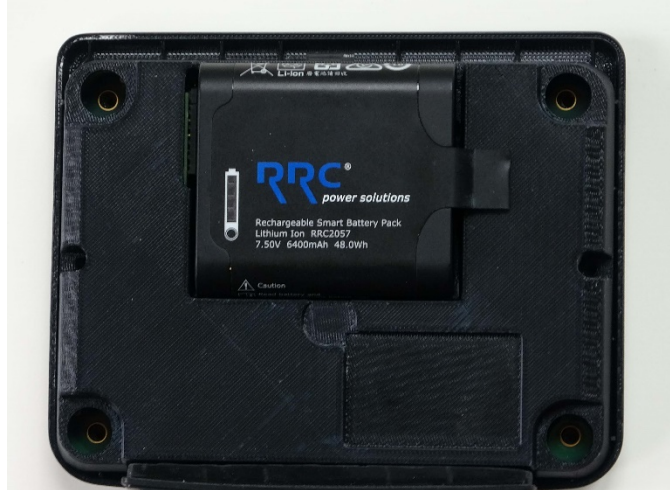
Figure 41: VentFree battery seated
