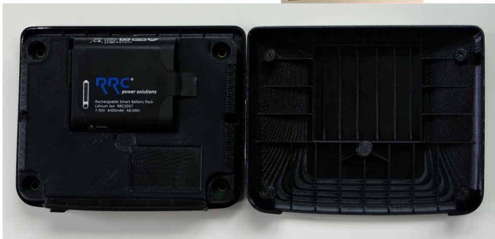
Figure 37: VentFree with back panel removed
