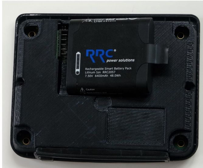
Figure 40: VentFree battery replaced
