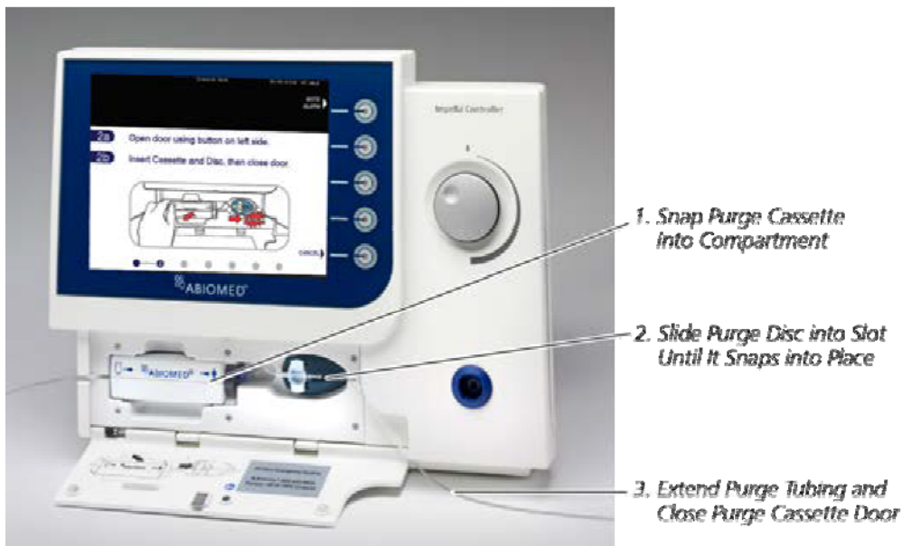
Figure 5.6 Inserting the Purge Cassette into the Automated Impella Controller
