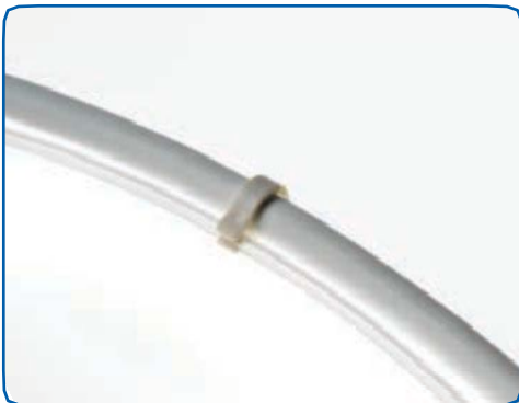
Figure 5.13 Connecting the Purge Tubing to the Connector Cable
