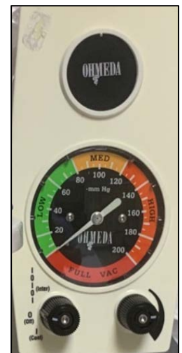
Figure 4 Wall mounted hospital regulator with suction pressure from 0 to 200 mm Hg.
