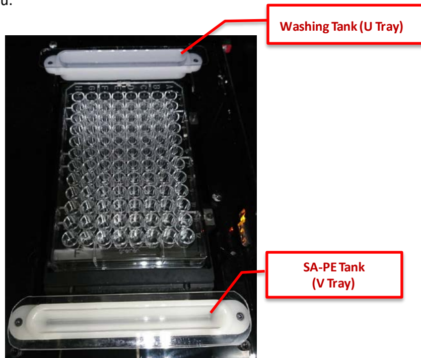
Fig. 27. Positions of the Washing and SA-PE Tanks
