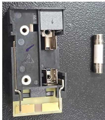
Fig. 41. Fuse and the fuse holder
