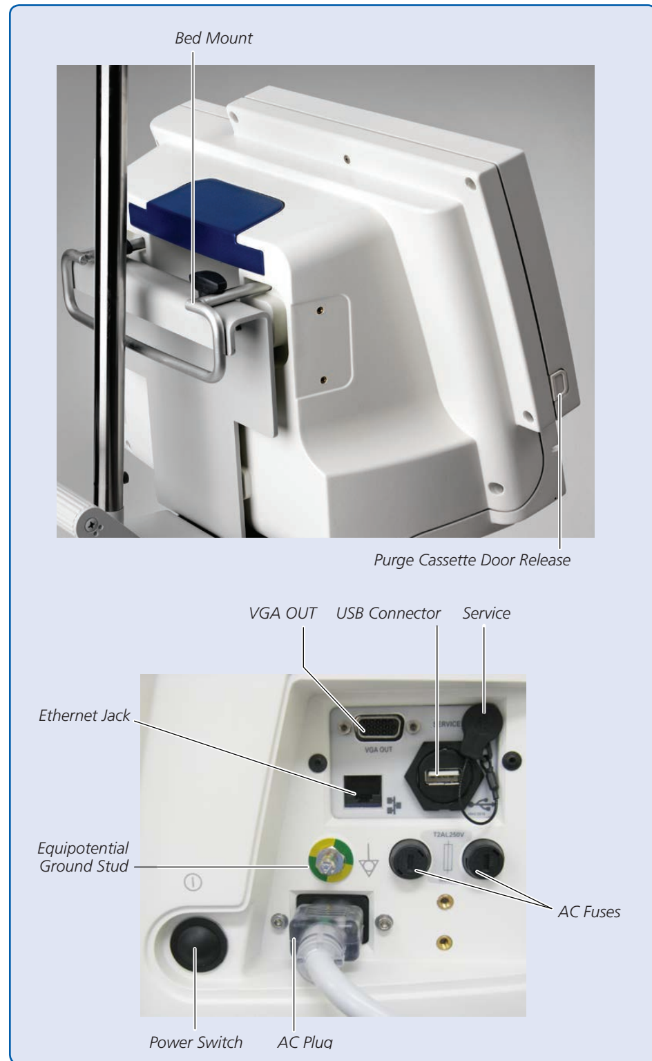
Figure 4.2 Automated Impella Controller Features – Side Views
