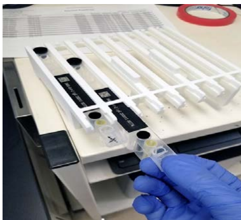
Figure 3: Inserting Controls Cartridges into Reagent Rack
