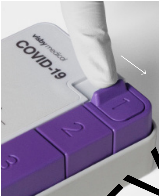
A After loading sample into device close button 1 by sliding the cap to the right.
