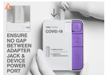
E Plug in the device until it clicks into place. A stable white light indicates the test is running. Ensure that there is no gap between the adapter jack and the device.
