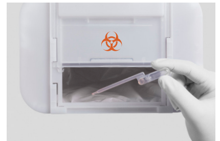
I Discard the Visby Pipette according to your institution's standard practices. Do not set it down . Recap the Visby Buffer Tube.
