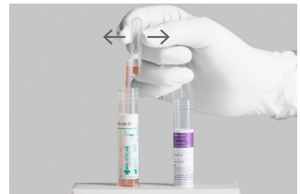
F Keep the tip fully under the fluid. Release the upper bulb.
