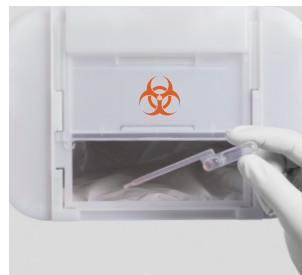
I Discard the Visby Pipette as per your institution's practices. Do not set it down.
