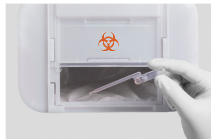
I Discard the Visby Pipette according to your institution's standard practices. Do not set it down. Recap the Visby Buffer Tube.
