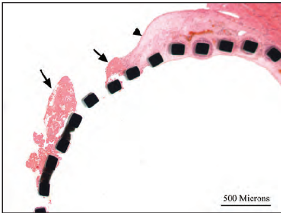
Figure 8. Thrombosis, score 1; Fibrin thrombus (arrows); Organized neointima (arrowhead). Animal 1039, Day 57, mid section, (H&E) 4x objective magnification.
