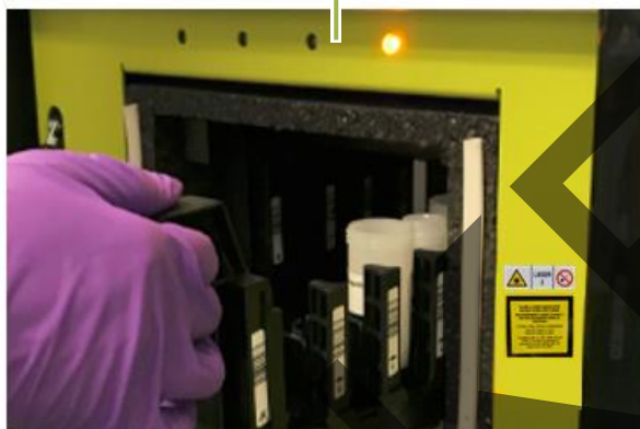
Reagent bay showing four reagent rack lanes
