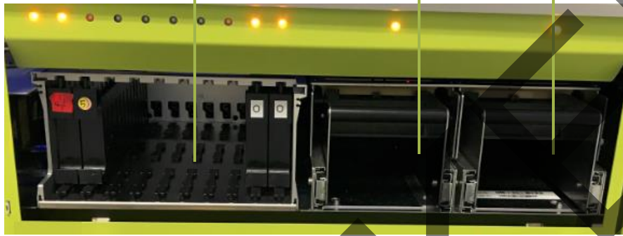
Sample bay, showing eight lanes for plate racks or tube racks and two lanes for RGP racks
