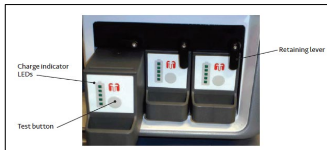
Figure 25: Removal of Discharged OCS™ Battery Pack
