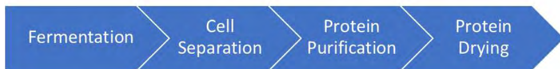
Figure 5: Overview of the manufacturing steps for NSEWP
