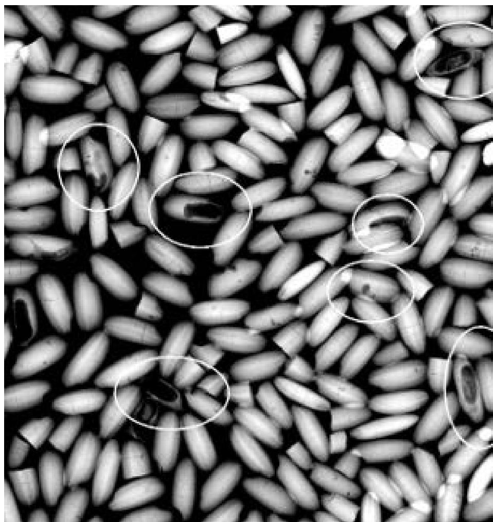
Figure V-3-A-34. X-ray of insect, Sitophilus sp. Schönherr, damaged basmati rice. Damage indicated by circles (3x). (Source: H. Loechelt-Yoshioka, FDA).
