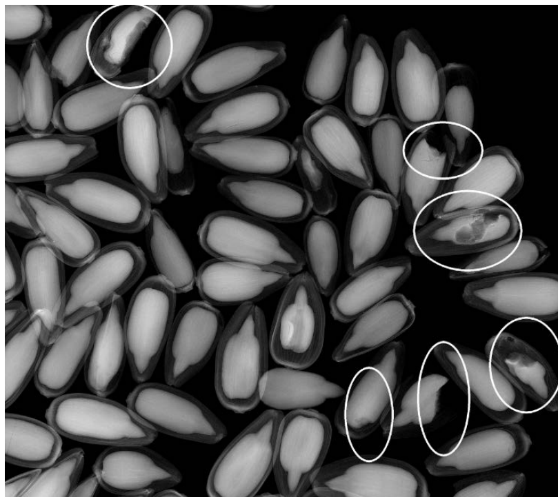
Figure V-3-C-12. X-ray image of sunflowers with hulls. Insect feeding damage indicated by circled seeds (3x). (Source: H. Loechelt-Yoshioka, FDA).
