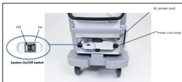
2. If necessary, unwind the power cord from the power cord wrap.
