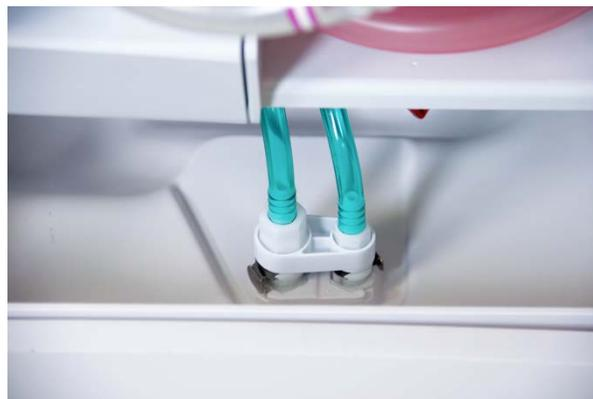
**NOTE**—To remove gas lines, pinch the metal tabs on each side of the bracket and lift connectors.
