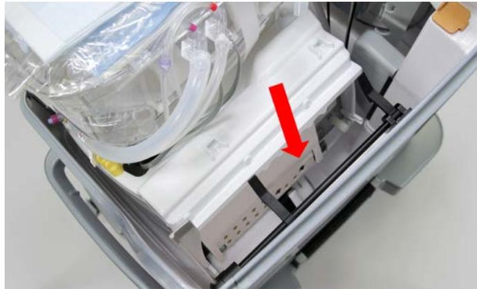
5. Maneuver the LvPM until the pump components slide into the grooves on each side of the locking ring.
