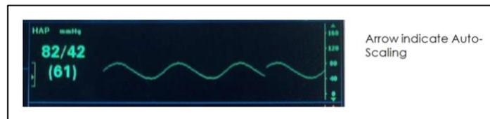
In manual scaling mode, the graph remains at one of the fixed scales that you configure by accessing the Actions Menu. When this mode is active, no arrow icons are displayed at the top and bottom of the y-axis scale.
