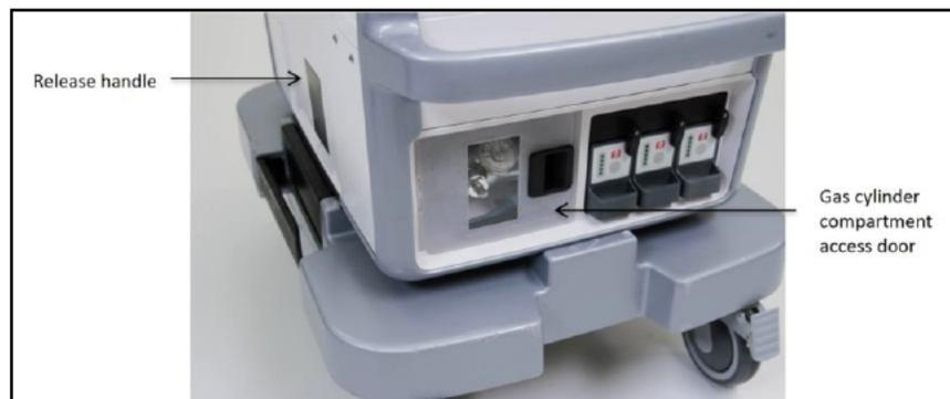
2. Open the access door to the gas cylinder compartment (Figure 68).
