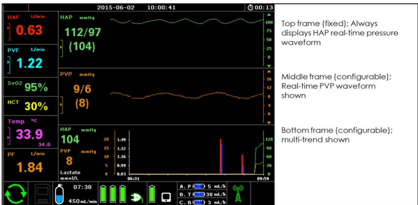
You can configure the middle and bottom graphical frames to display either real-time pressure waveforms or trend data. Each time you change modes during the session, the graphical frames that you configure for that mode are automatically displayed on the Wireless Monitor. For detailed instructions, see Section 10.5, “Configuring Session Settings.”
