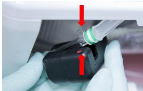
3. Snap the probe into place around the cuvette.
