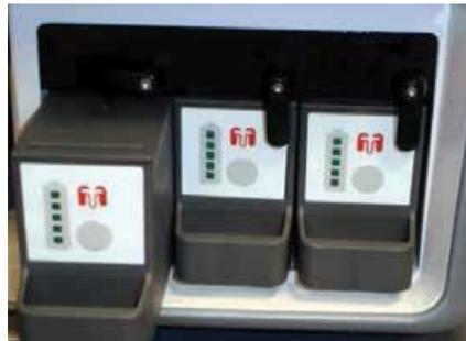
The OCS™ batteries (Figure 14) are installed in the battery compartment on the right side of the Liver Console, next to the gas cylinder compartment, as shown in Figure 4. When the OCS™ is connected to AC power, the batteries automatically charge.
