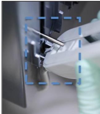
4. While fully squeezing the SDS Cassette’s attachment fingers, firmly press the SDS Cassette onto the SDS Console’s pressure sensor.
