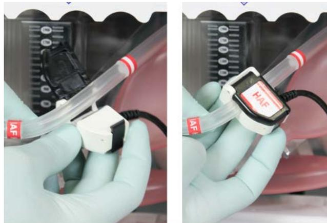
6. Make sure the lid is completely closed and the latch is secure. The fit should be tight, with the full tubing cross-section contacting all inner surfaces of the sensing window. The tubing will be slightly compressed into a rectangular shape.
