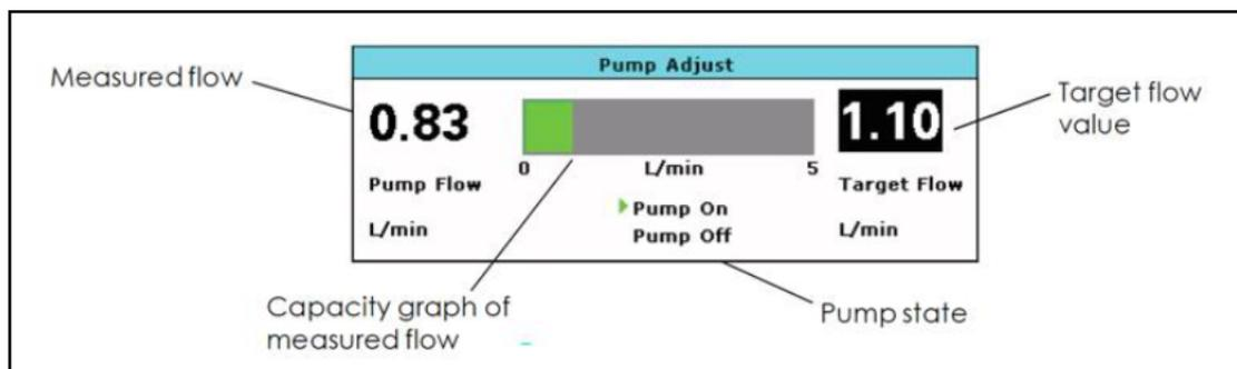
**CAUTION**— Perfusate warming, SDS infusion, and gas flow are enabled only when the pump is on (and if the pump becomes faulted). Setting the pump to OFF turns off the circulatory pump, SDS infusion, the gas, and the blood warmer. When the pump flow is off, physiological parameter alarm monitoring is disabled.
