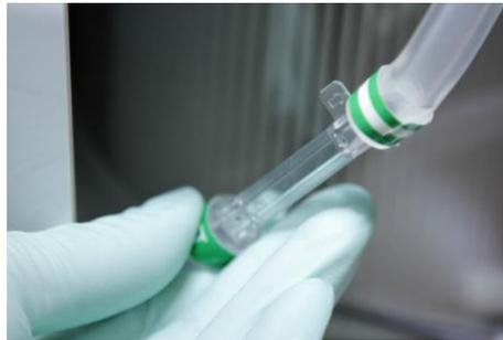
2. Align the SvO<sub>2</sub>/HCT Probe so that the cuvette is centered in the probe opening (use the single and double green bands on the probe and the tubing to position it properly). Also align the red dot on the probe with the tab on the cuvette.
