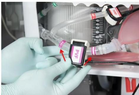
2. Open the probe cover by pressing down on the black latch to release it (Figure 35).
