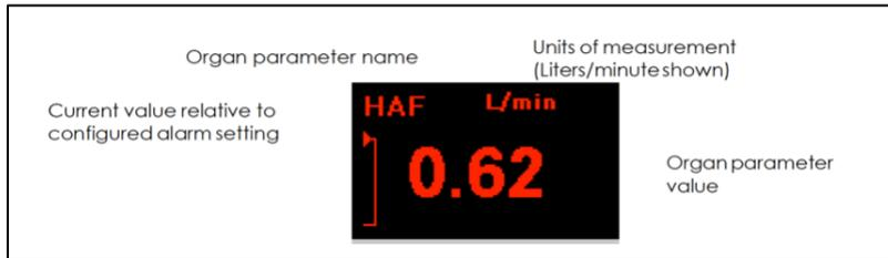
The value of each organ parameter is also displayed with an arrow (to the left of the value) to indicate its location relative to the upper and lower alarm limits, or relative to the total parameter range if there is no upper or lower limit.
