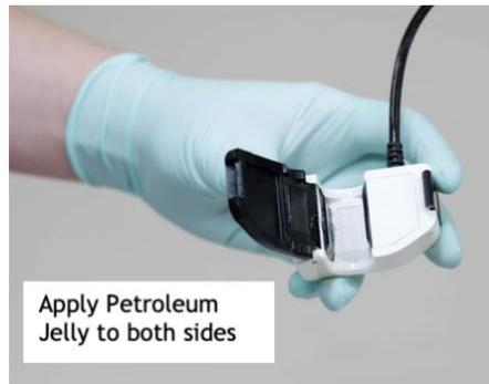
**CAUTION**—Use only petroleum jelly. Any other coupling gel, such as silicone grease or ultrasound gel, may damage the probe.
