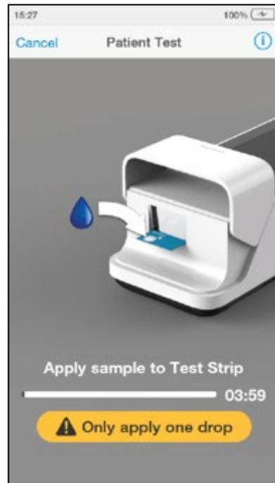
When the sample is detected the Instrument will sound and a confirmation message will be displayed.
