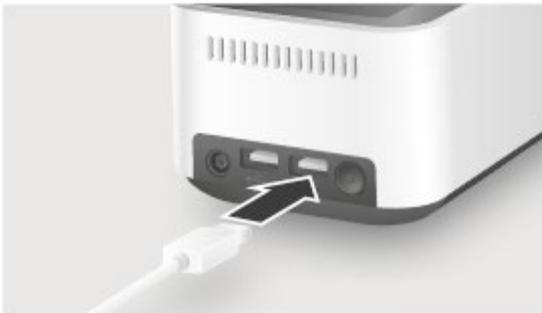
Insert USB connector into one of the USB ports at the rear of the Instrument.
