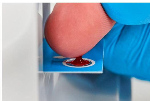
When the sample is detected, the Instrument will sound and a confirmation message will be displayed.
