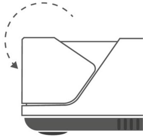
3. **Do not open the door while the test is in progress.** The touch-screen will indicate test progress.
