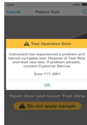
**Example of an error screen:** If the On Board Control (OBC) fails, an error message will be shown and no test result will be returned. Follow the on screen instructions to dispose of the Test Strip and start a new test. If the problem persists, contact Customer Services.
