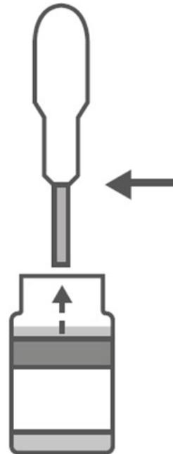
2. **Apply the Quality Control solution to the already inserted SARS-CoV-2 Ab Test Strip.** Hold the pipette over the Sample Application Area of the Test Strip and dispense the Quality Control solution. The LumiraDx Instrument will indicate sample is detected with an audible alert (if the Instrument sounds are enabled). The screen of the LumiraDx Instrument will request the user to close the door. Dispose of pipette.
