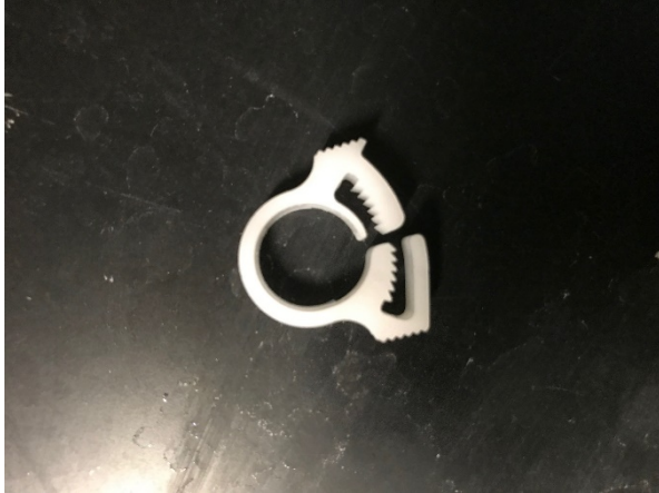
Photo 1. Hose clamp (Cole-Parmer # 6832-04; Min ID: 0.402", Max ID: 0.449")
