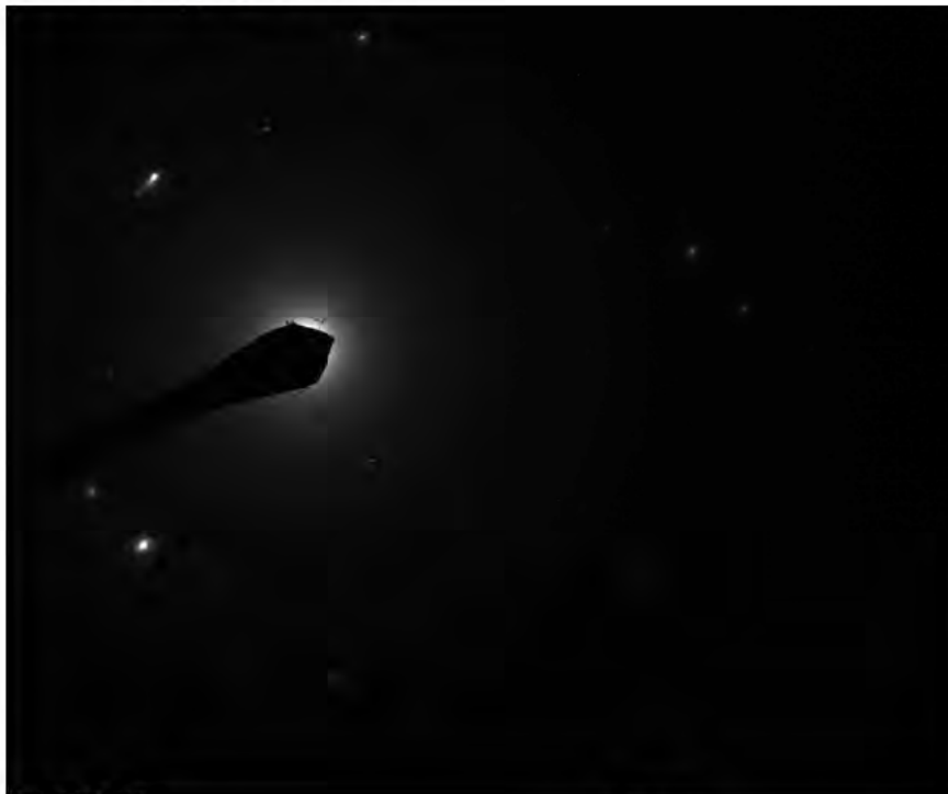
621000 FDA_128.jpg Iron Fiber 14:52 4/21/2020 TEM Mode: Diffraction Microscopist: (b)(6) Camera: NANOSPR15, Exposure: 800 (ms) x 5 drift frames, Gain: 1, Bin: 1 Gamma: 1.00, No Sharpening, Normal Contrast
