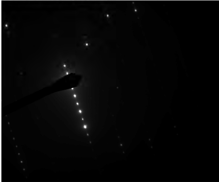
621000 FDA_092.jpg Structure 4 13:13 4/17/2020 TEM Mode: Diffraction Microscopist: [b](6) Camera: NANOSPRT5, Exposure: 800 (ms) x 5 drift frames, Gain: 1, Bin: 1 Gamma: 1.00, No Sharpening, Normal Contrast
