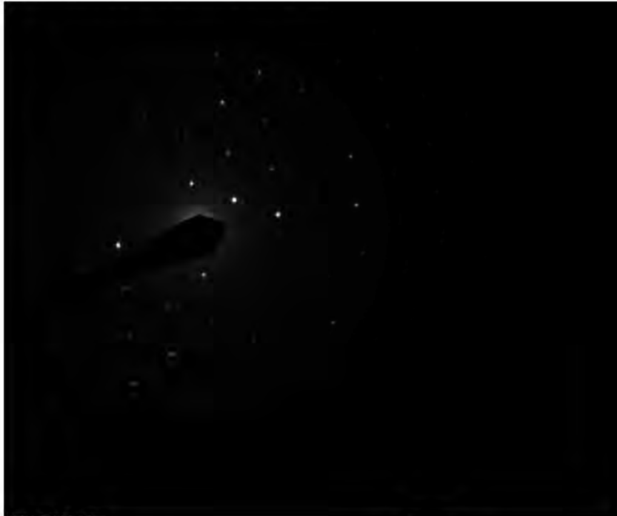
621000 FDA_082.jpg Mica Fiber 12:08 4/17/2020 TEM Mode: Diffraction Microscopist: (b)(6) Camera: NANOSPRT5, Exposure: 800 (ms) x 5 drift frames, Gain: 1, Bin: 1 Gamma: 1.00, No Sharpening, Normal Contrast
