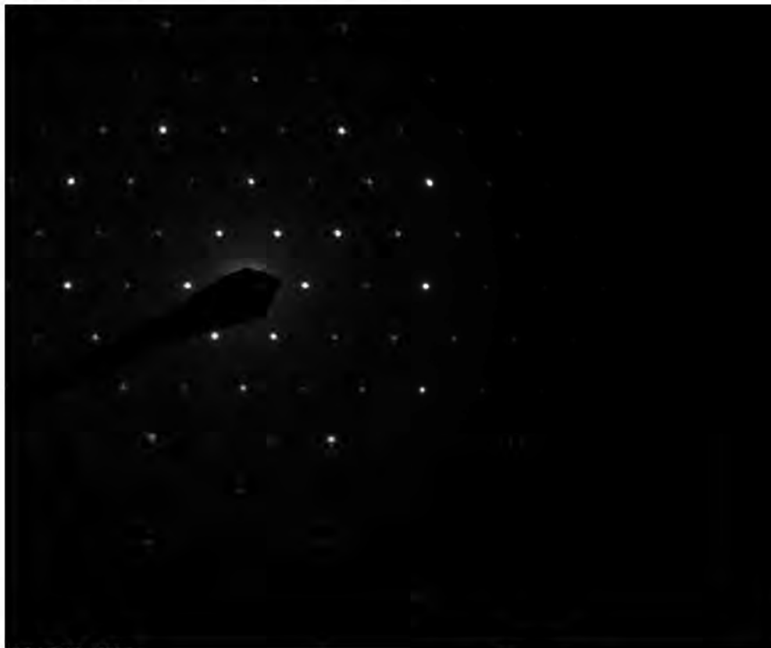
621000 FDA_119.jpg Talc Fiber 13:18 4/21/2020 TEM Mode: Diffraction Microscopist: (b)(6) Camera: NANOSPR15, Exposure: 800 (ms) x 5 drift frames, Gain: 1, Bin: 1 Gamma: 1.00, No Sharpening, Normal Contrast
