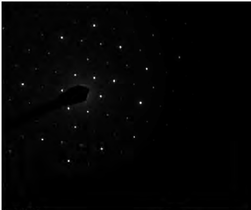
621000 FDA_153.jpg Talc Fiber 11:27 4/22/2020 TEM Mode: Diffraction Microscopist: (b)(6) Camera: NANOSPR15, Exposure: 800 (ms) x 5 drift frames, Gain: 1, Bin: 1 Gamma: 1.00, No Sharpening, Normal Contrast
