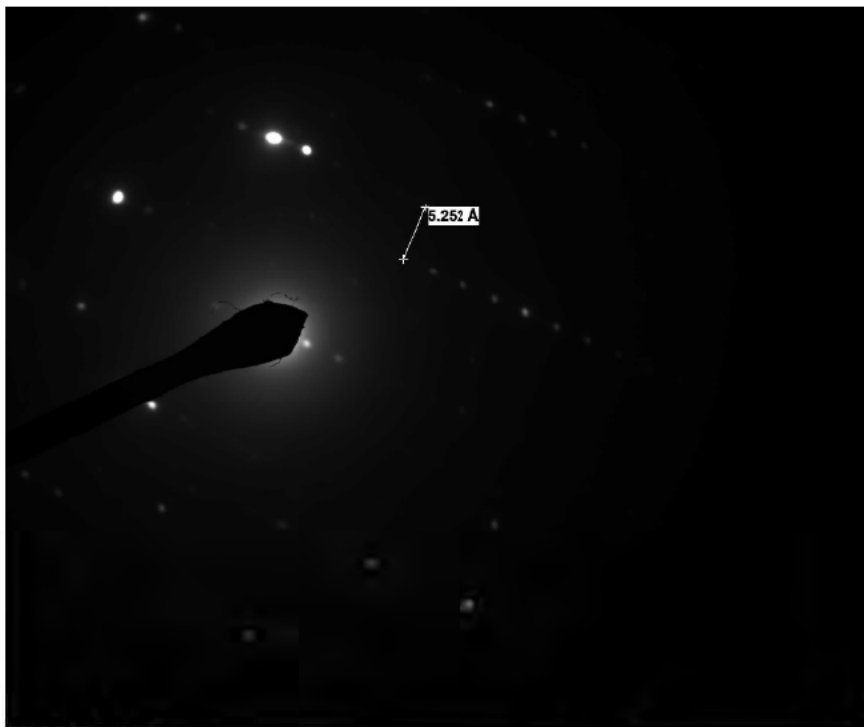
621000 FDA_067.jpg Structure 1 11:19 4/17/2020 TEM Mode: Diffraction Microscopist: (b)(6) Camera: NANOSPRT5, Exposure: 800 (ms) x 5 drift frames, Gain: 1, Bin: 1 Gamma: 1.00, No Sharpening, Normal Contrast
