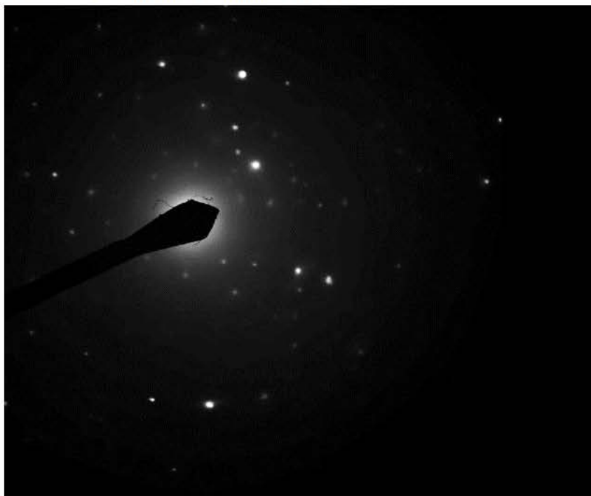
Diffraction Pattern from the Particles Containing Titanium pictured above
