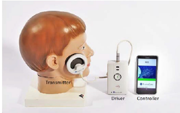
Figure 5 Energy Delivery and Control (EDC) Set
