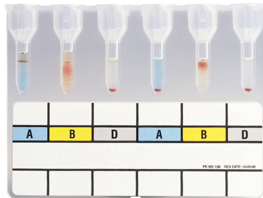
MTS™ A/B/D Monoclonal Grouping Card: Group AB Rh-negative and Group B Rh-negative are shown
