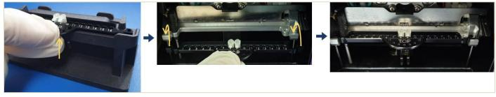
9.05.05) Unlatch the metal flap by raising the black hook, this will allow the sprint-loaded metal flap to go back to its pressing position.
