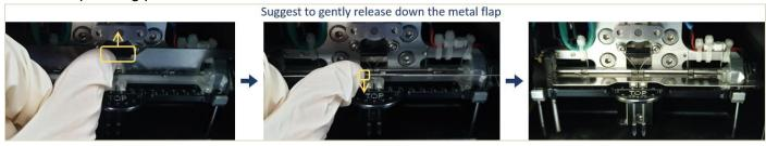
9.05.06) To unload capillary / rack, open the front door, then flip up the metal flap till it is latched.
