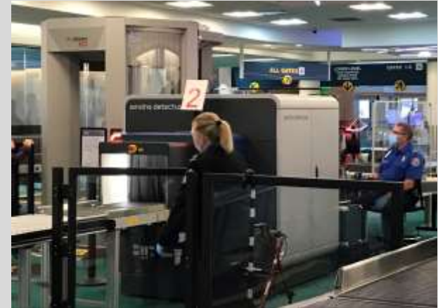
3D – computed tomography airport baggage scanner
