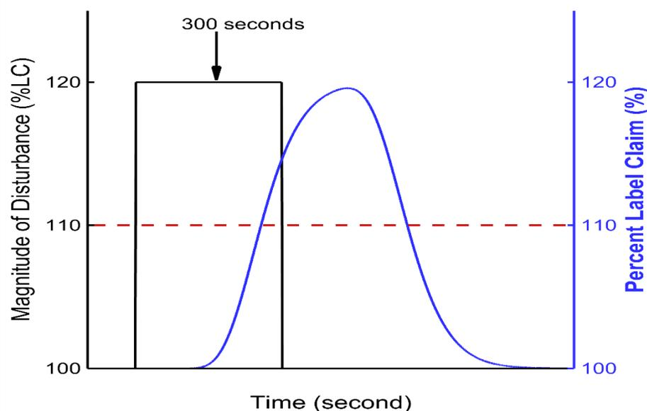
**Description:** Figure 7 illustrates a drug substance LIWF with an unexpected transient +20 percent flow spike lasting 300 seconds. The disturbance is outside the predefined acceptance criteria for disturbances. This disturbance causes an increase in the amount of the drug substance fed into the blender before returning to normal operating condition. The funnel plot (Figure 5) shows that following this disturbance, the drug substance concentration in the blend exceeds the
