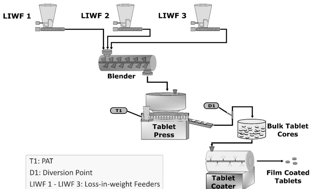
A PAT tool using an NIR method monitors blend uniformity and triggers tablet diversion. Run time at a predefined mass flow rate is used to define the batch size range; in this case, the overall marketing demand requires batch sizes between 360 and 1080 kilograms of the drug product.
