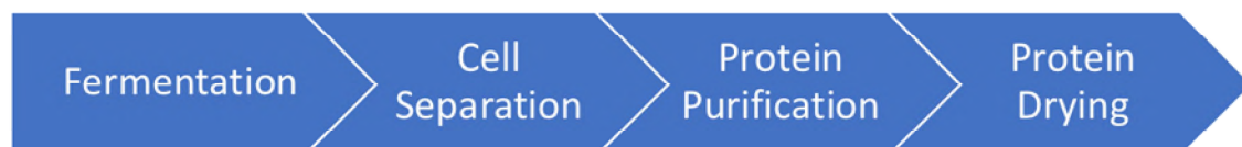
Figure 5. Overview of the manufacturing steps for NEWP
