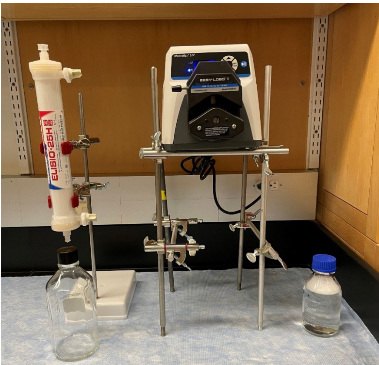
Fig. 16. The filter is secured vertically using the stand clamps with the sample inlet port pointing downwards, and the effluent side port oriented towards the pump.
