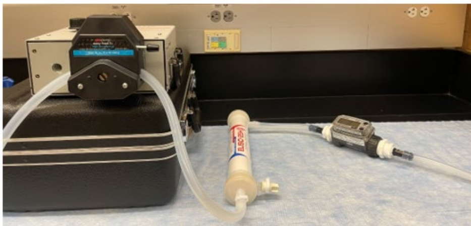
Fig 12. Appropriate configuration of effluent tubing and water flow meter.
