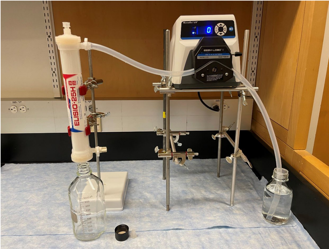
Fig. 17. During the filter set up, the sample inlet port points downwards, and the effluent side port faces the pump. The sample receiving bottle is placed under blood return port without touching the bottle surfaces. The tubing is attached to the dialysate outlet port by pushing onto the port and is secured with a SNP-12 clamp or a zip tie.
