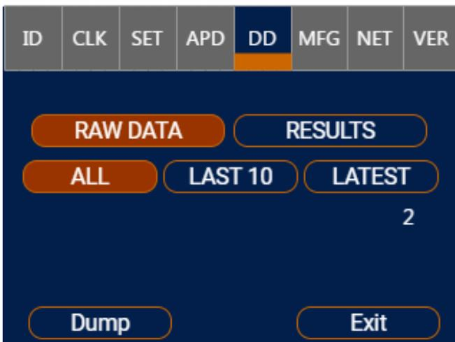
➤ Press the **“DD”** tab. This will display the data dump screen. Select **“RESULTS”** or **“RAW DATA”**. The number of runs available to download will be displayed above the exit button. You must select **“ALL”** and press **“DUMP”** to download all data from the instrument.
