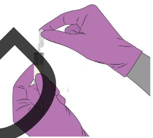
Squeeze **top bulb** of pipette over the **Reagent Container** to discharge all fluid from pipette shaft. Some fluid will still remain in the bottom bulb of the pipette.
