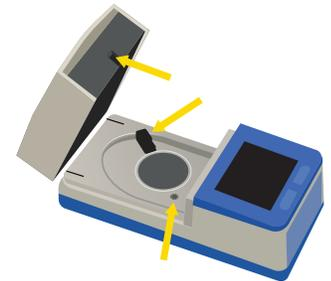
⚠ Take caution to avoid touching the temperature sensors and light pipe during cleaning.
