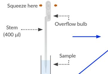
Release top bulb to fill the entire pipette shaft until fluid enters the overflow bulb. **Visually confirm that the entire shaft is filled with fluid before proceeding.** **Note:** Do not invert the Transfer Pipette when filled with fluid. If there is a bubble formed when drawing up fluid, or if no fluid enters the overflow bulb, discard and re-try with a new pipette.
