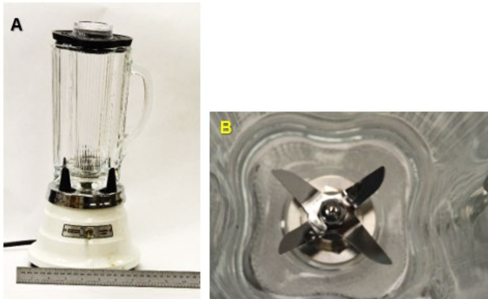
Figure II-1. A. High speed blender, Waring blender B. Close-up view of the canted stainless-steel blades. (Source: Photos courtesy of H. Loechelt-Yoshioka, FDA).
