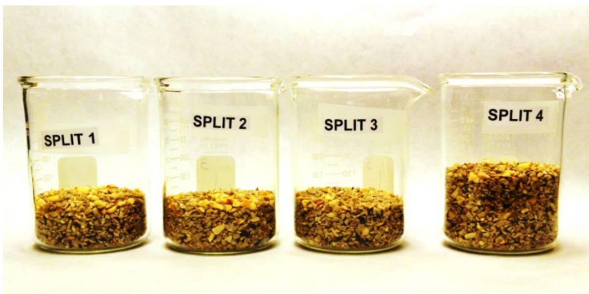
Figure II-10. Fractional Shoveling. Splits 1-3 are correct and split 4 is incorrect. (Source: Photo courtesy of H. Loechelt-Yoshioka, FDA)
