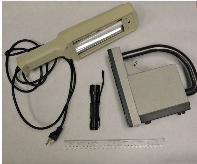
Figure II-31. Examples of different UV light sources. (Source: Photo courtesy of H. Loechelt-Yoshioka, FDA).
