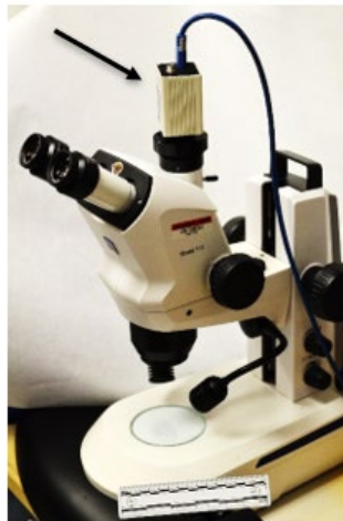
Figure II-20. An example of a stereomicroscope with attached camera indicated by arrow. (Source: Photo courtesy of H. Loechelt-Yoshioka, FDA).
