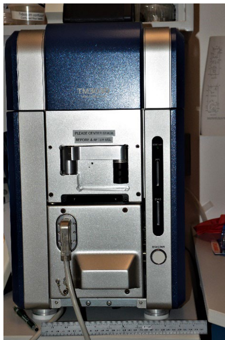
Figure II-22. Bench Top Scanning Electron Microscope (SEM). (Source: Photo courtesy of H. Loechelt-Yoshioka, FDA).
