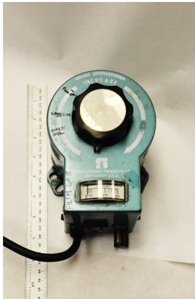
Figure II-2. Variable Speed Transformer. (Source: Photo courtesy of H. Loechelt-Yoshioka, FDA).
