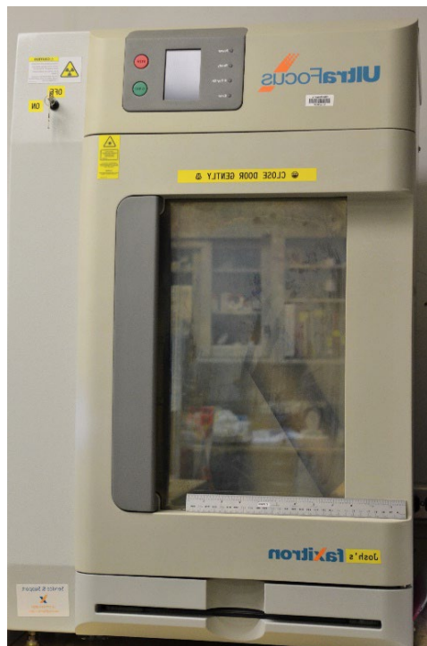
Figure II-32. Example of a bench top X-ray machine. (Source: Photo courtesy of H. Loechelt-Yoshioka, FDA).
