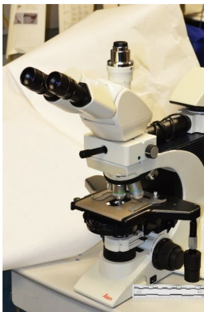
Figure II-21. An example of a compound microscope. (Source: Photo courtesy of H. Loechelt-Yoshioka, FDA).
