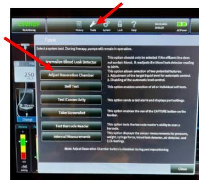
**Figure 42:** Location of 'Tools' button and 'Adjust Deaeration Chamber' button
