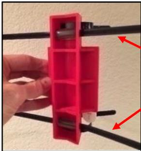
Figure 25: The pre-attached zip-ties are used for securing the SCD-PED Cartridge to the front of the bracket after the SCD Securing Bracket has been previously mounted to the side of the CKRT machine (refer to Section B, Step 1 for bracket mounting).
