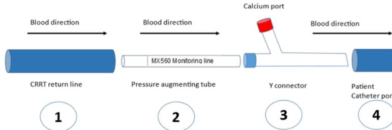
Figure 24: Connection location of MX560 (a) and diagram of connections (B)
