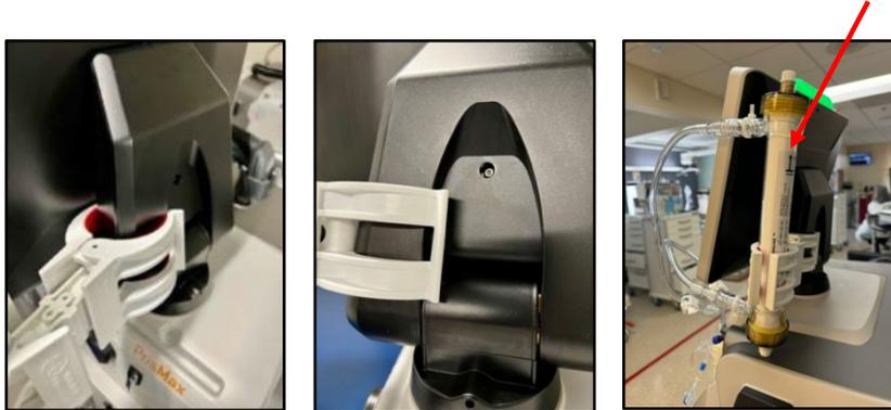
**Figure 34: The SCD Holder has two identical clamps (one that clamps to the side of the monitor's base, and the other clamp for holding the SCD-PED Cartridge).**
