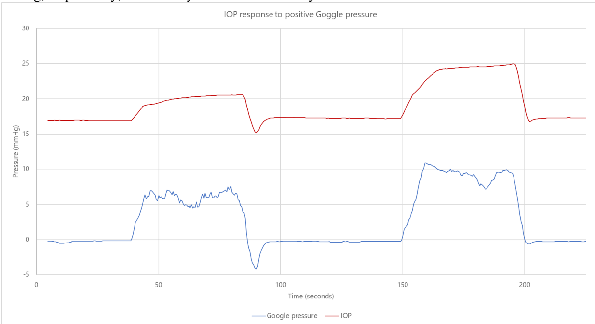
Figure 3: Application of +5 mmHg and +10 mmHg results in an average increased IOP of 3mmHg and 7mmHg, respectively, in a directly cannulated full body cadaver.
