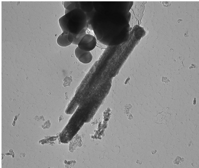
646090-14, Elongated Particle Containing Chromium and Iron
