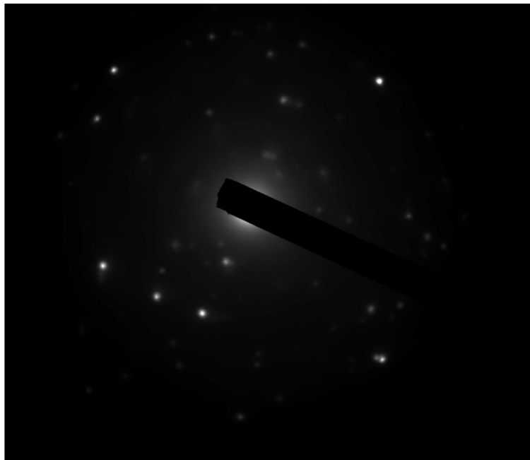
647186 FDA_092.jpg 647186-9 Fe particles FDA Cal: 0.000477 \mu\text{m}/\text{pix} 11:10 2023-08-23 TEM Mode: Diffraction Microscopist: (b) (6) Camera: NS6, Exposure: 500 (ms) x 3 drift frames, Gain: 1, Bin: 1 Gamma: 1.00, No Sharpening, Normal Contrast 0.2 \text{\AA}^{-1} HV=80kV Cam Len: 0.2000 m
