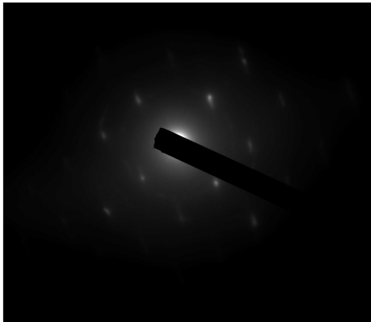
647186 FDA_115.jpg 647186-11 Talc ribbon FDA Cal: 0.001612 \mu\text{m}/\text{pix} 11:38 2023-08-28 TEM Mode: Diffraction Microscopist: (b) (6) Camera: NS6, Exposure: 500 (ms) x 3 std. frames, Gain: 1, Bin: 1 Gamma: 1.00, No Sharpening, Normal Contrast 0.2 \text{\AA}^{-1} HV=80kV Cam Len: 0.2000 m
