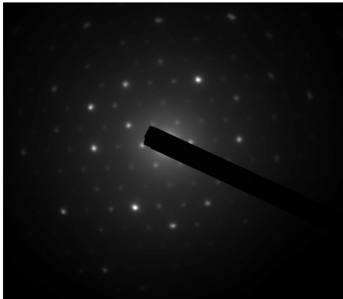
647186 FDA_137.jpg 647186-13 Talc FDA 11:57 2023-08-29 TEM Mode: Diffraction Microscopist: (b) (6) Camera: NS6, Exposure: 500 (ms) x 3 std. frames, Gain: 1, Bin: 1 Gamma: 1.00, No Sharpening, Normal Contrast 0.2 \text{\AA}^{-1} HV=80kV Cam Len: 0.2000 m
